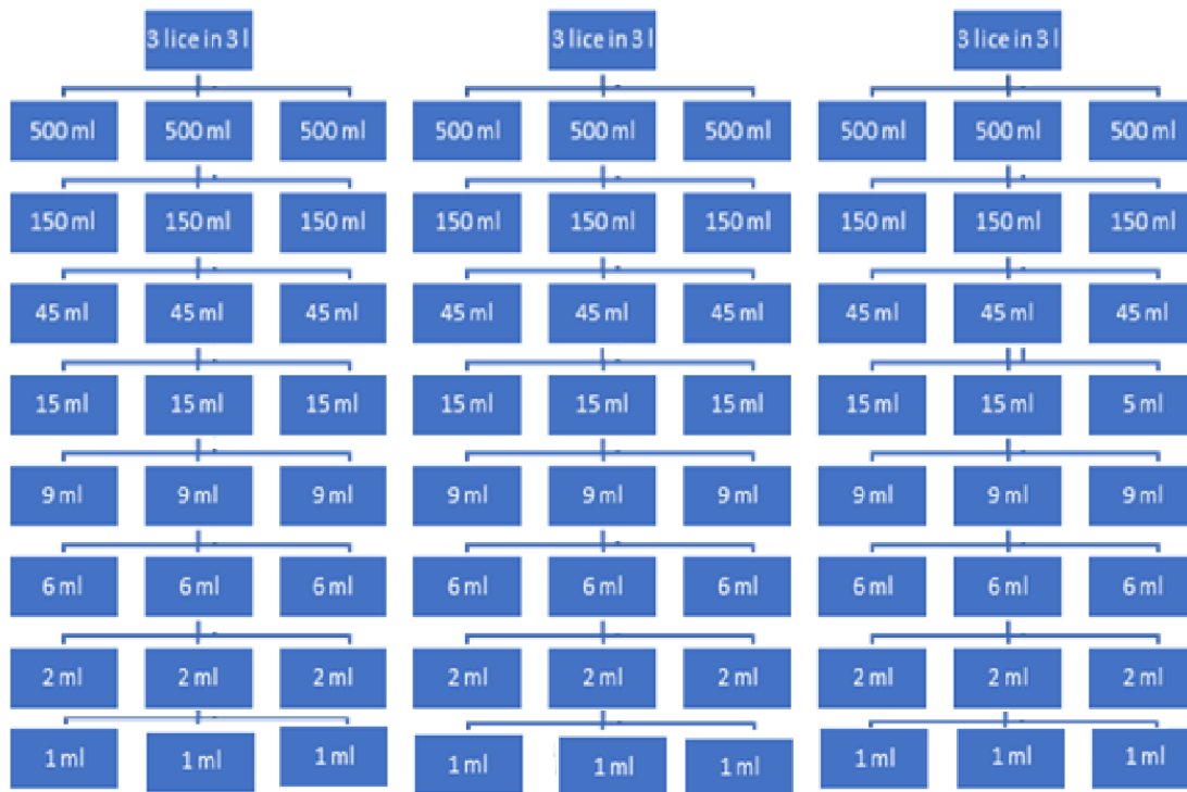
Figure 6 Dilution setup, all blue squares represents a 3 L can. The three top ones contained 3 salmon lice in 3 L of water each and were used as reservoir for “salmon lice water” which were added to the cans below. The ones below the three “reservoirs” contained the given amount of added salmon lice water to achieve a total volume of 3 L.
