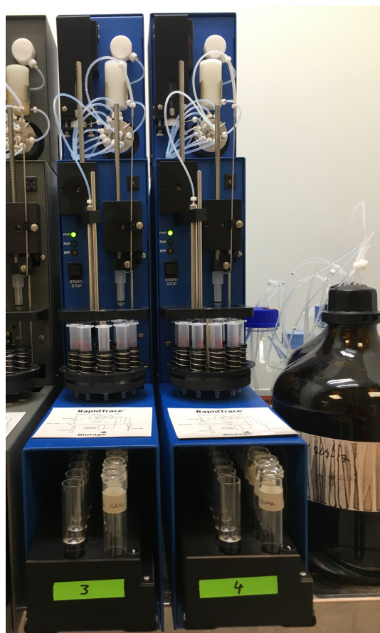
Figure 27: SPE robot. In the modules (3 and 4) fraction collection tubes are placed to the left and samples to the right. Florisil packed columns are stored above the modules, and a cannula transfers solvents and sample through the column to the fraction collector. The robot worked over night, and this picture was taken next morning. The sample fractions (left in modules) have at this point evaporated a little.
