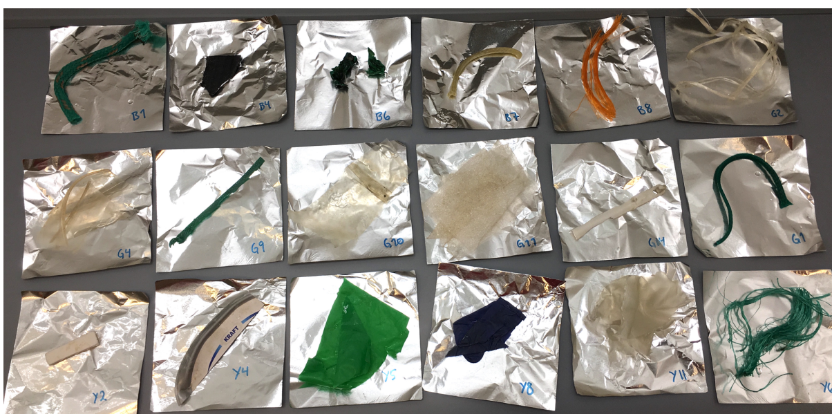
Figure 26: 18 out of 28 plastic garbage items collected along the shoreline in Longyearbyen. These were cut into microplastic pieces and analysed for POPs. Random sample id name can be seen in lower, right corner at each aluminium sheet. Colour and density varies among samples.
