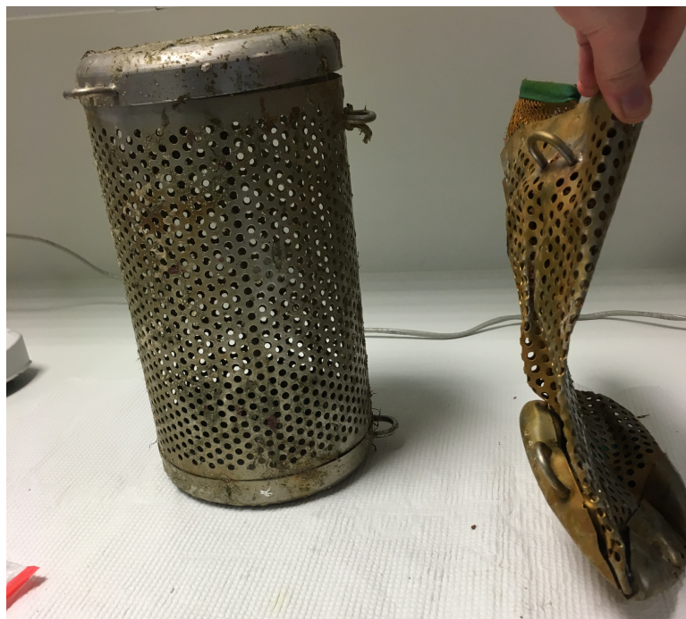
Figure 30: Sample holding containers from the summer batch (left) and the winter batch(right). The green fabric that can be seen in the winter container belongs to the washing net holding the samples inside the container, which was completely stuck.
