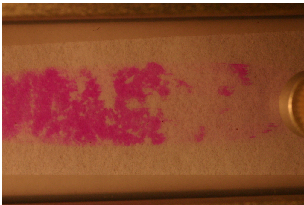
Figure 4.25: Photograph taken of the AF4 channel, six minutes after the elution step began for a fractionation of 100 \mu\text{g} Rh-PE liposomes.
