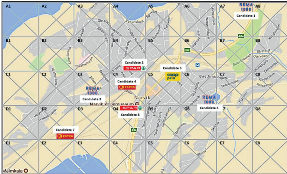
FIGURE 4: Customer demand aggregation and candidate locations for postal service counters.
