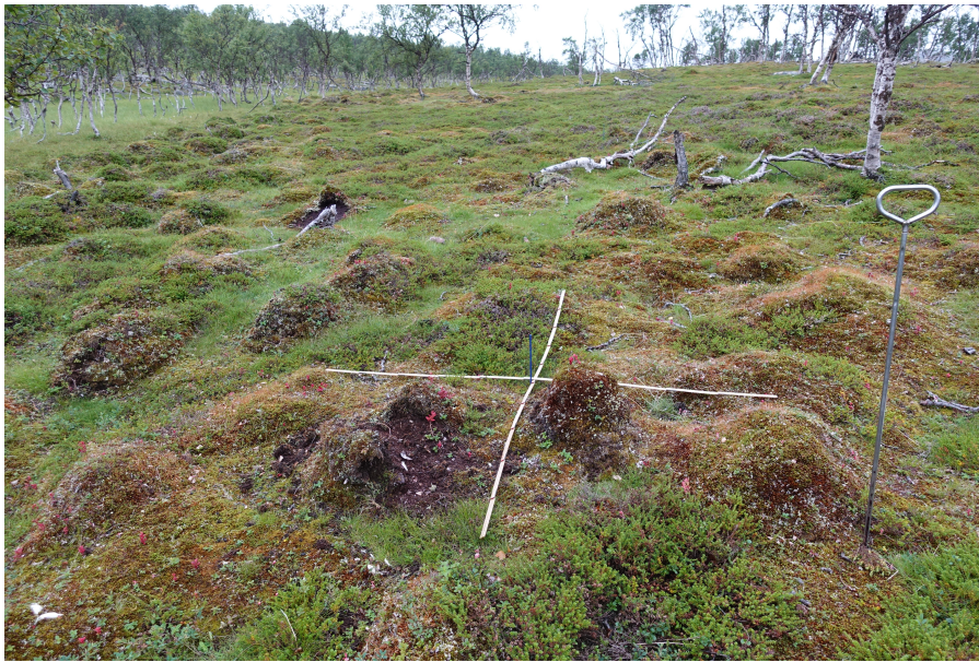
Figure 3.5: Image of a point for soil depth measurements, using metersticks of 2 meter to find 1 m distance from the center.
