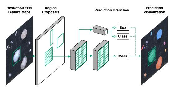
Figure 4. Simple, sketch-like depiction of the Mask R-CNN model architecture.
