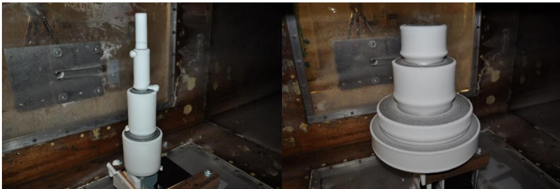
Figure 12 – Final ice shapes of the small (left) and large (right) cylinder configurations in the Cranfield University icing tunnel experiments.
