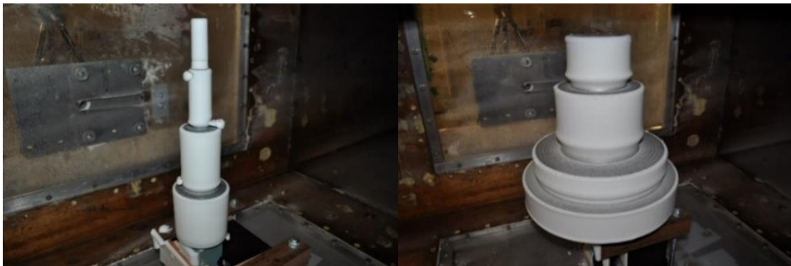
Fig. 1 – Final ice shapes of the small (left) and large (right) cylinder configurations.
