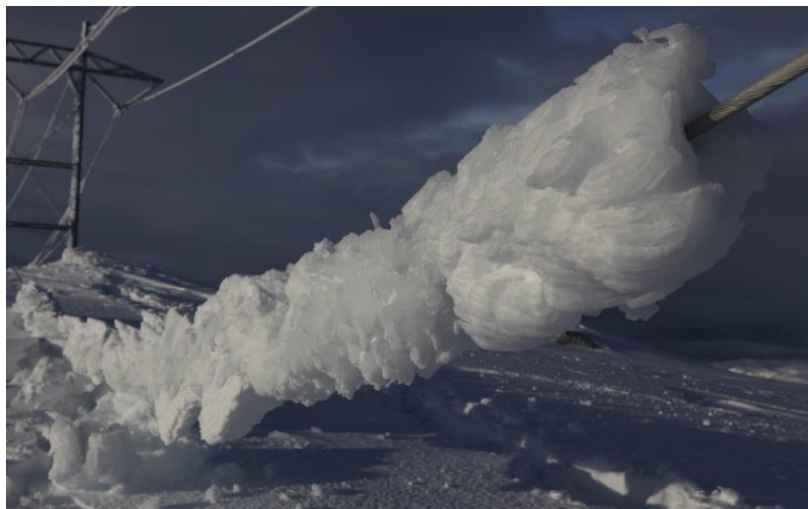
Figure 1 – Accumulated rime ice on a broken ground wire, January 2014. An ice load of 68 kg/m was estimated based on its diameter and an ice density sample (Nygaard et al., 2017). (Photo: Ole Gustav Berg, Statnett).
