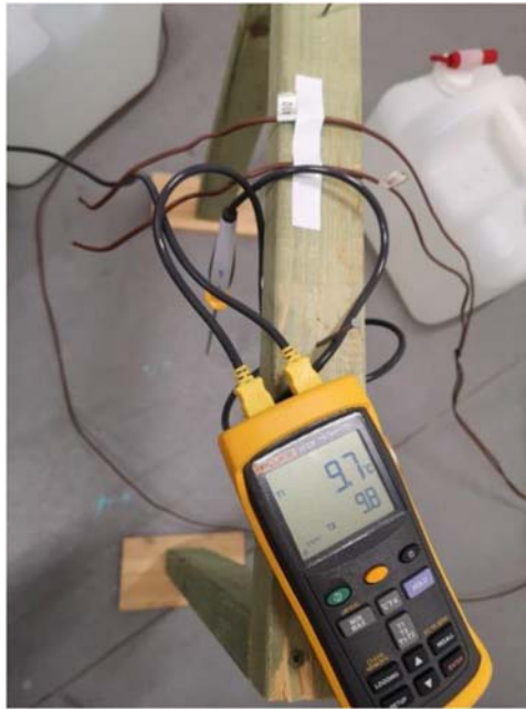
Picture 7. The Fluke 54 II B thermometer and probes measuring air temperature, taped to a wooden rail. The photo was taken during the test performed at +10°C.
