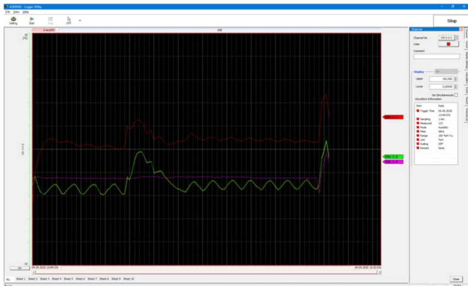
Figure 6. Hioki logger plot output showing the disturbance in temperature caused by cooling cycles and entering and exiting the test facility.
