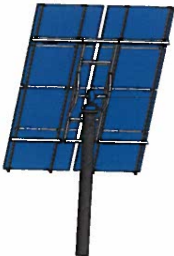
Fig. 1 Solar panel rig with two-axis orientation
