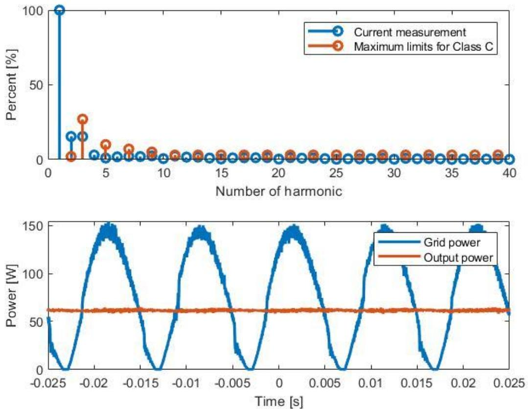
Figure 59. Harmonic content, maximum limits for Class C equipment according to IEC 61000-3-2 and power tested for the first converter at the second test.
