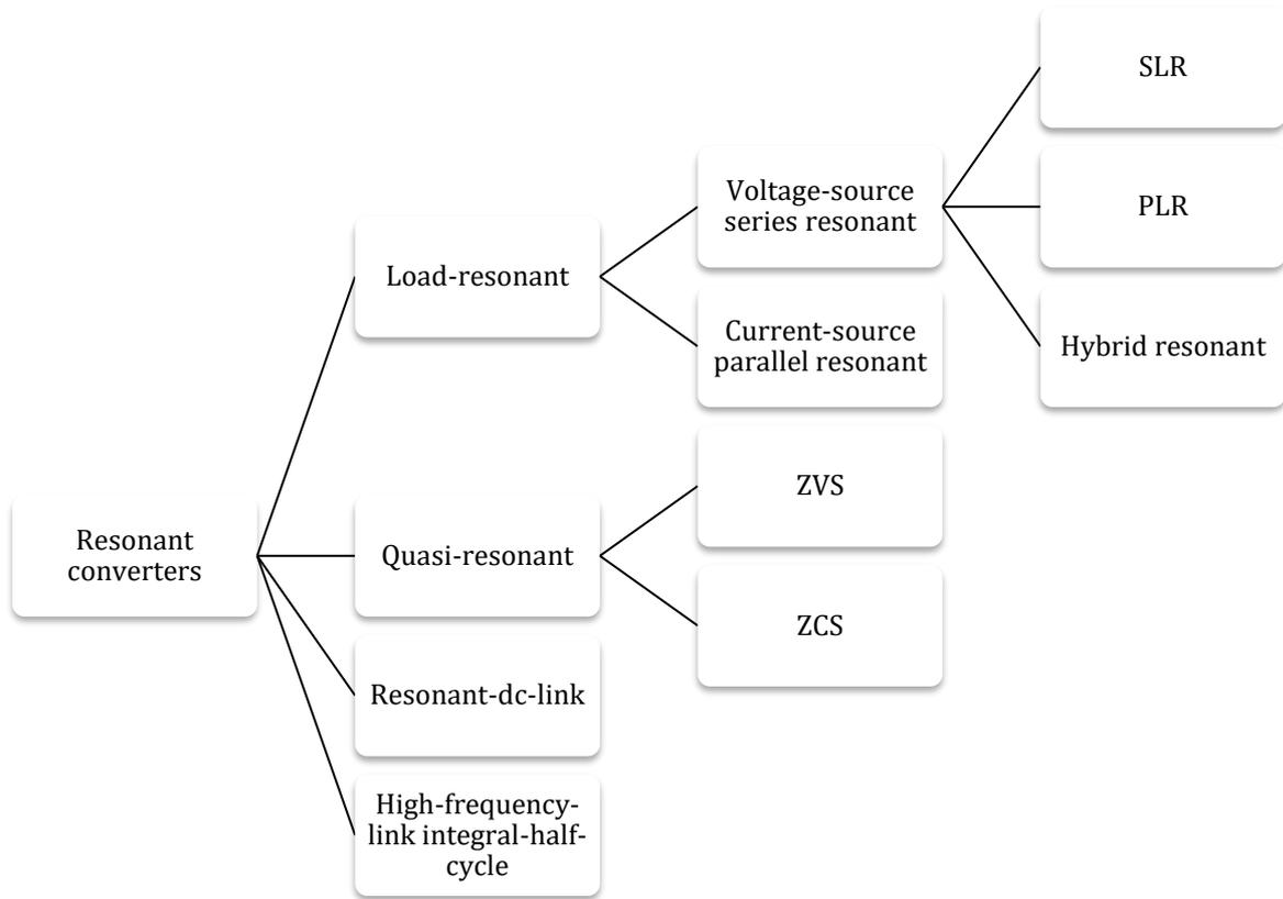
Figure 11. Resonant converters divided into Load-resonant converters, Quasi-resonant converters, Resonant dc-link converters and high-frequency-link integral-half-cycle converters.
