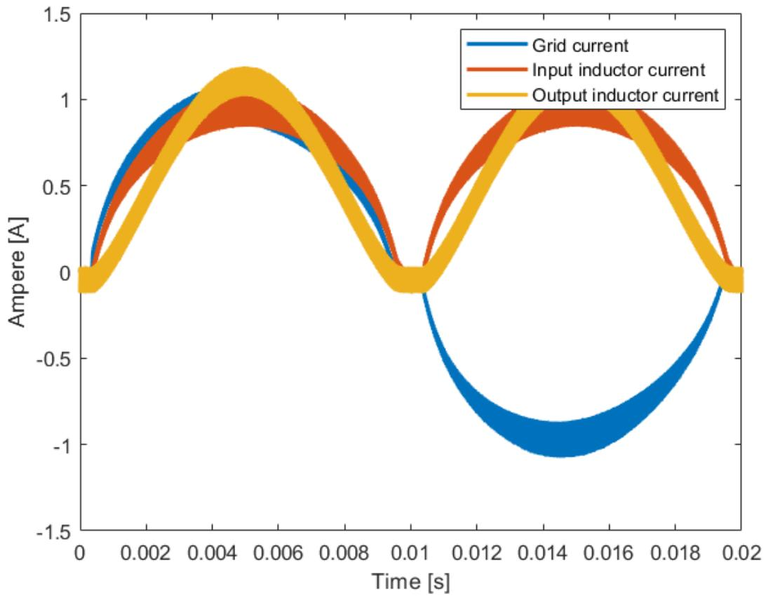
Figure 36. Simulation of grid current, input inductor current and output inductor current for the second suggested converter.
