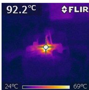
Figure 48. Temperature measured on the transistor during testing of the first suggested converter at 120 V/ 60 Hz.
