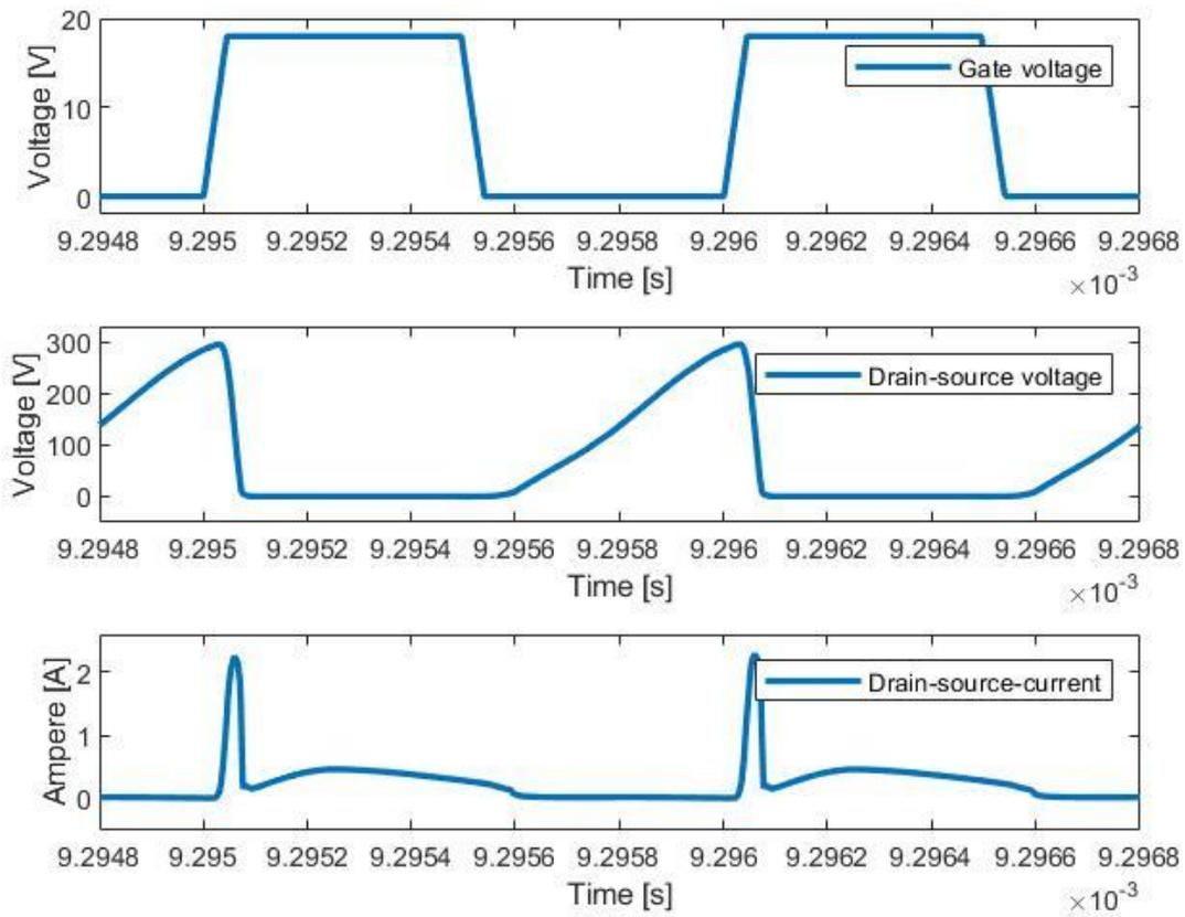
Figure 34. Simulated result of gate voltage and drain-to-source voltage and current during low voltage across the transistor for the first suggested converter.
