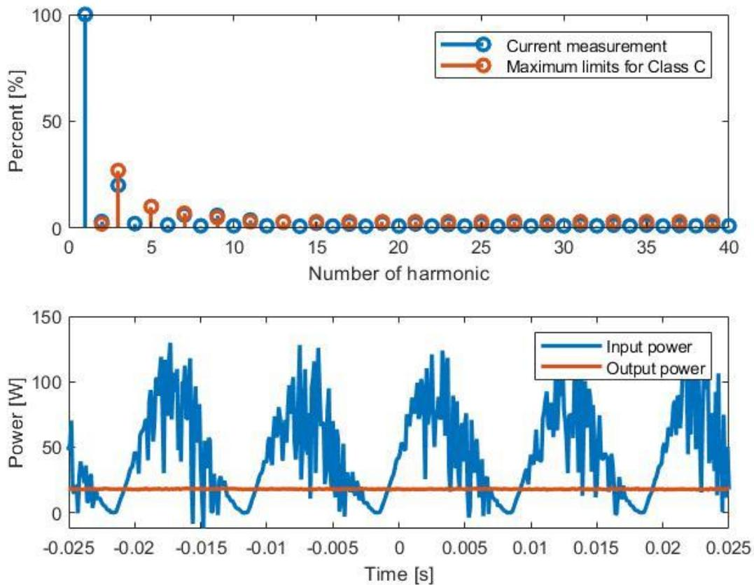
Figure 43. Harmonic content, maximum limits for Class C equipment according to IEC 61000-3-2 and power tested for the first converter at 240 V/ 50 Hz.
