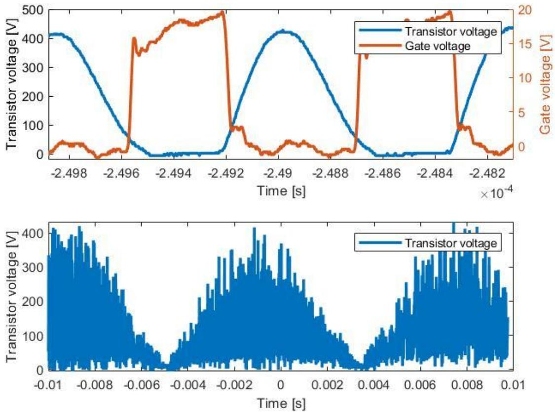
Figure 64. Drain-to-source and gate voltage across switching cycles and drain-to-source voltage across line cycle for the first converter at the second test for 120 V/ 60 Hz.
