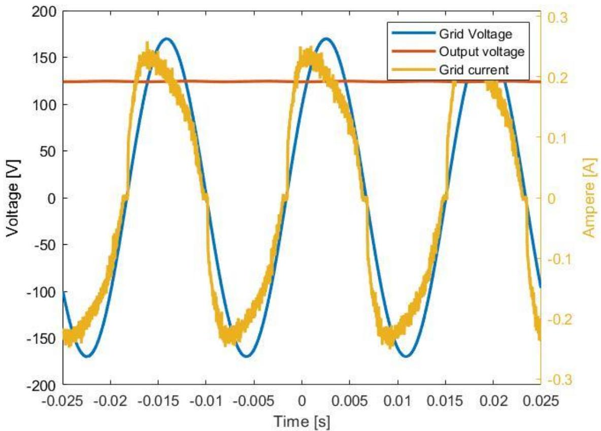
Figure 62. Grid voltage, output voltage and grid current for the first suggested converter at the second test of 120 V/ 60 Hz.
