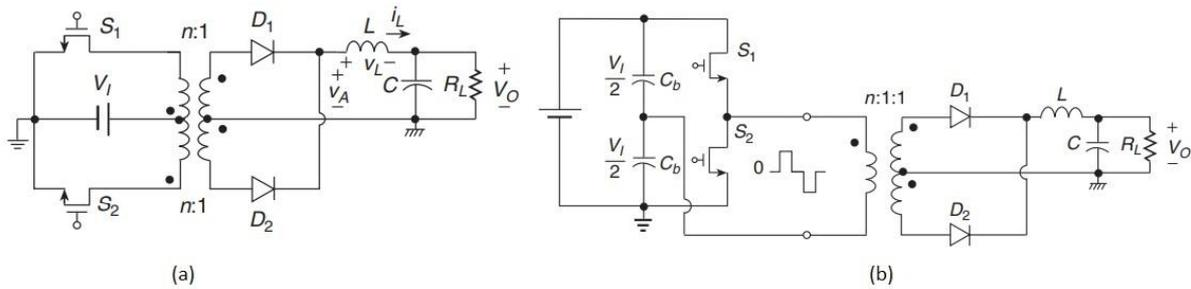
Figure 10. Push-pull and half bridge topology: (a) A push-pull converter. (b) A half-bridge converter topology [6].
