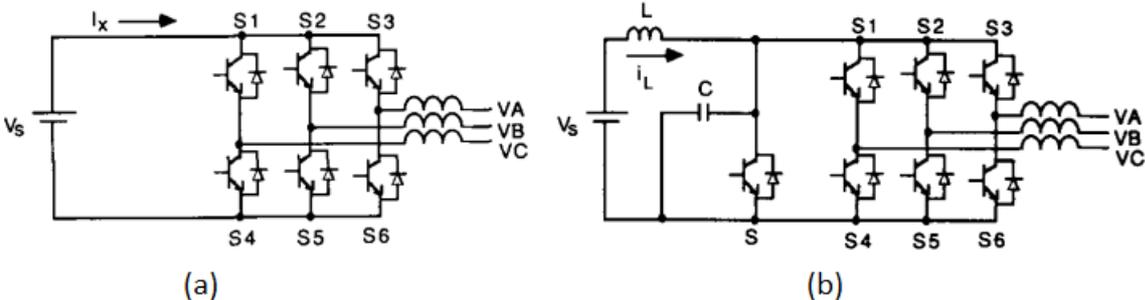
Figure 15. Conventional PWM and Resonant DC-link converter: (a) Conventional PWM converter. (b) Resonant DC-link converter topology [26].
