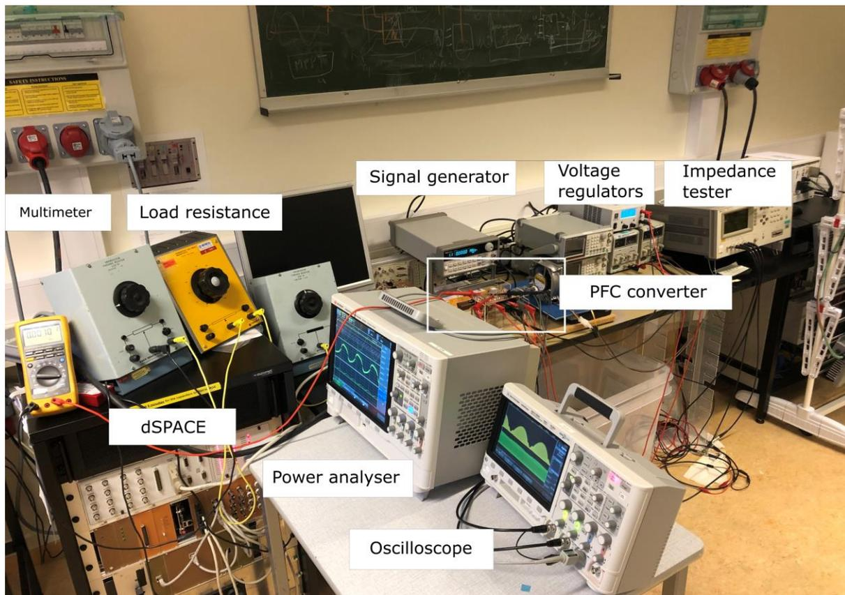
Figure 41. Equipment used through testing of converters.
