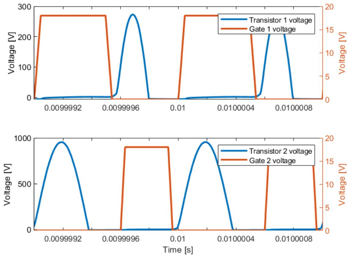
Figure 39. Simulation of ZVS across two switching-cycles for second suggested converter during low drain-to-source voltage.
