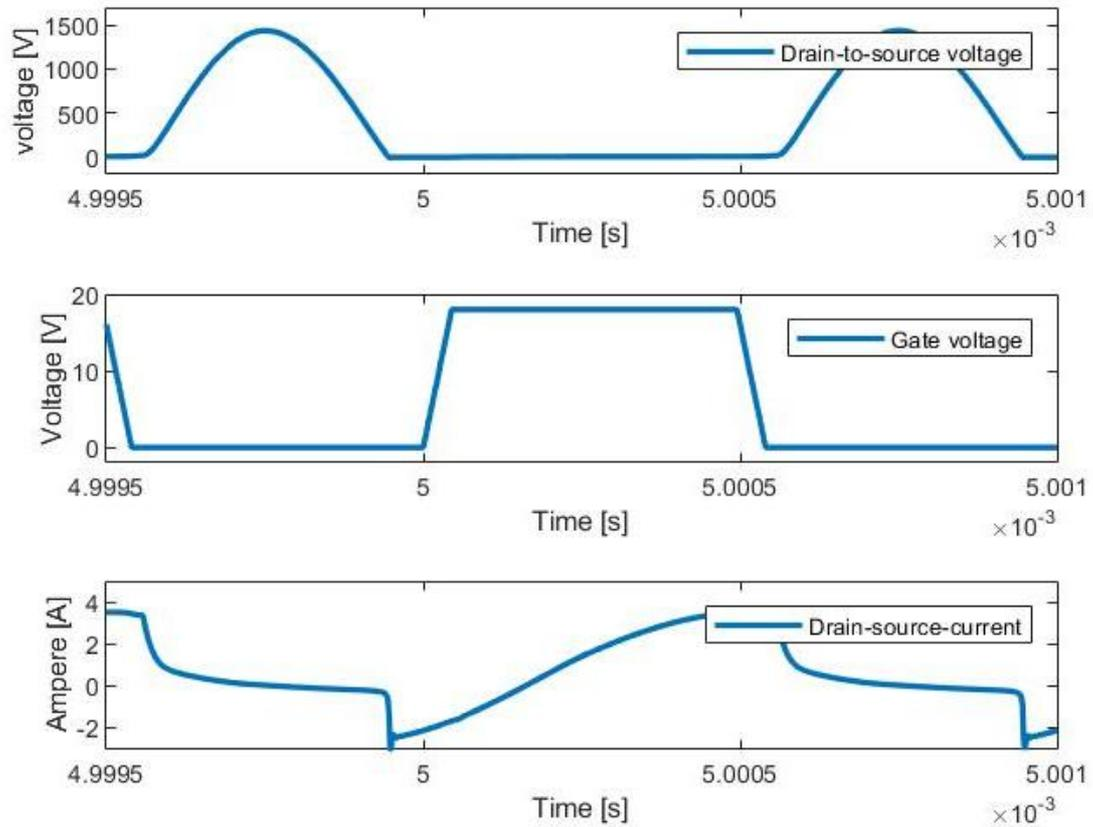
Figure 30. Simulation of drain-to-source voltage, gate voltage and drain-to-source current for the first converter.
