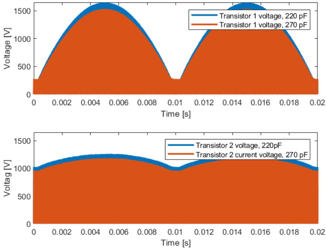
Figure 40. Simulation of a comparison between drain-to-source voltage and current across line-cycle with 220 pF and 270 pF shunt capacitor for the second suggested converter.
