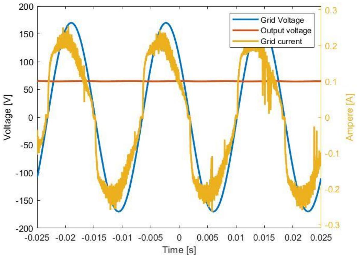
Figure 46. Grid voltage, output voltage and grid current for the first suggested converter at 120 V/ 60 Hz.
