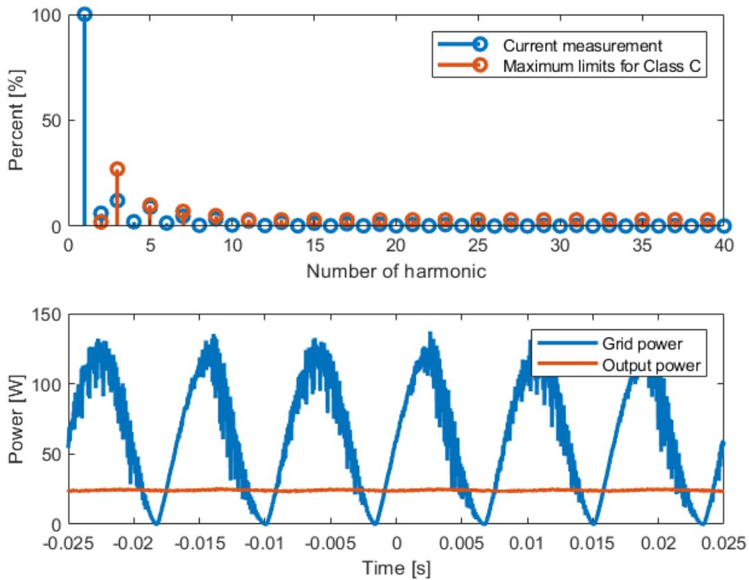
Figure 50. Harmonic content, maximum limits for Class C equipment according to IEC 61000-3-2 and power tested for the second converter at 120 V/ 60 Hz.
