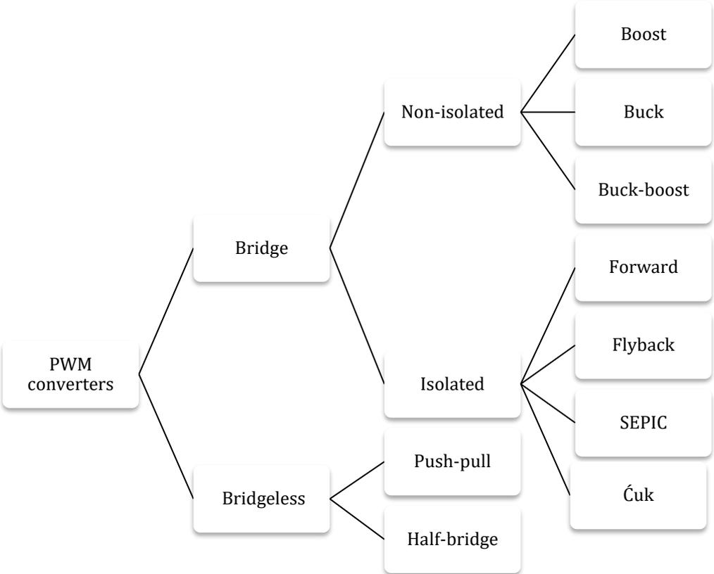
Figure 7. PWM converter divided into bridge and bridgeless converters.
