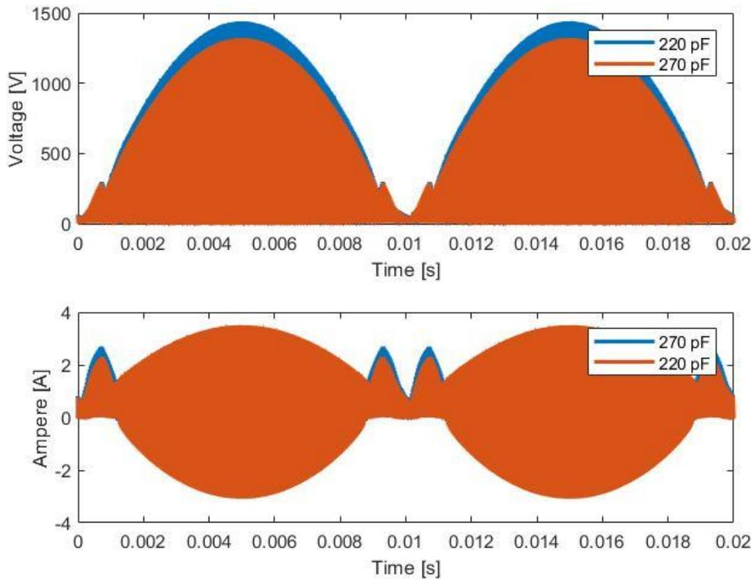
Figure 32. Difference in drain-to-source voltage and current when changing the shunt capacitor from 220pF to 270pF for the first suggested converter.
