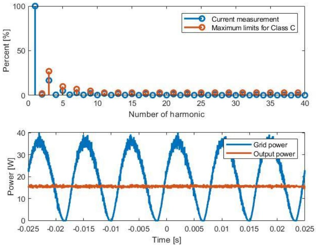
Figure 63. Harmonic content, maximum limits for Class C equipment according to IEC 61000-3-2 and power tested for the first converter at the second test for 120 V/ 60 Hz.
