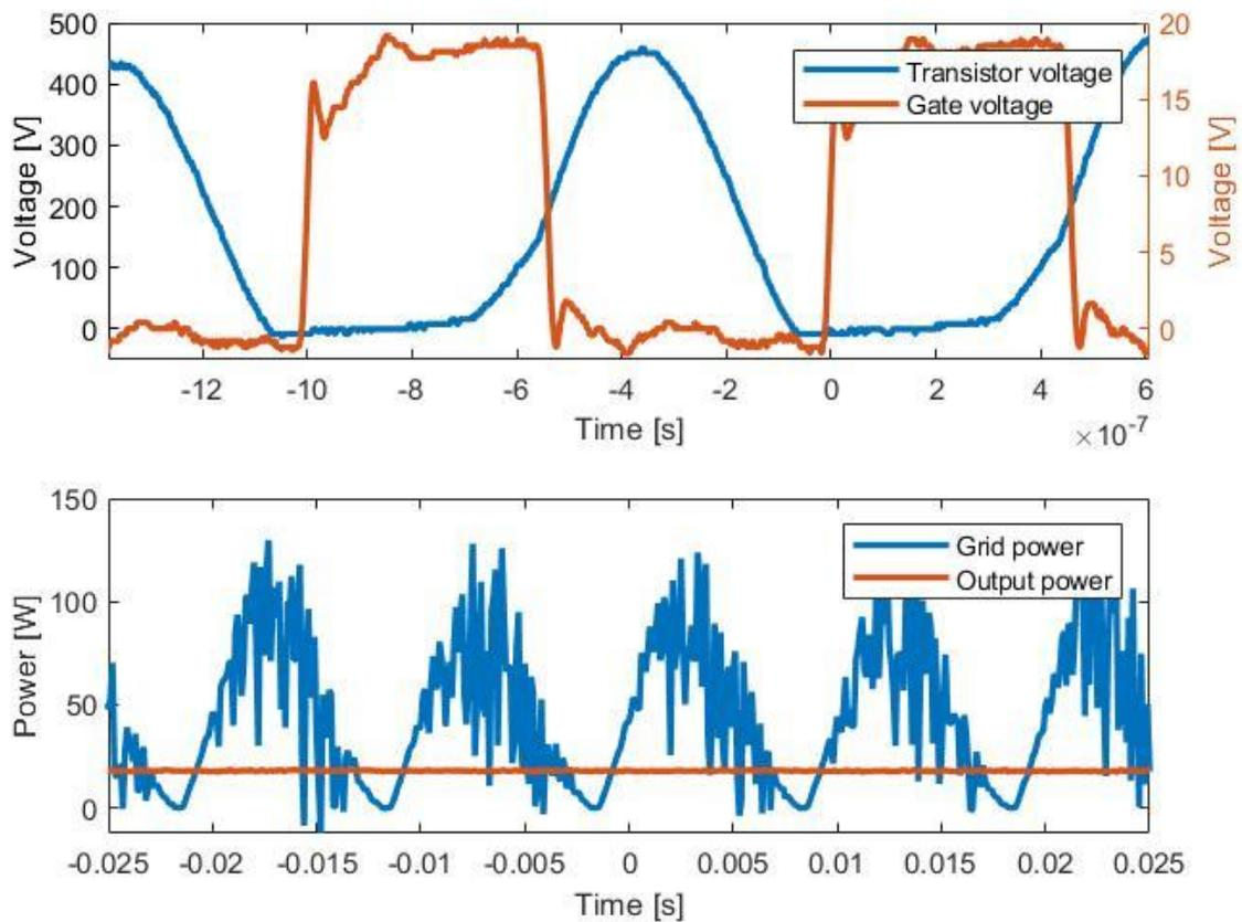
Figure 47. Drain-to-source and gate voltage across switching cycle and power across line cycle for the first suggested converter at 120 V/ 60 Hz
