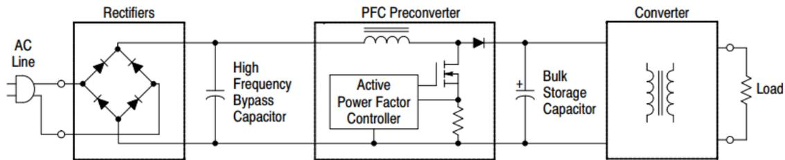
Figure 2. Offline AC-DC converter with power factor correction [4].
