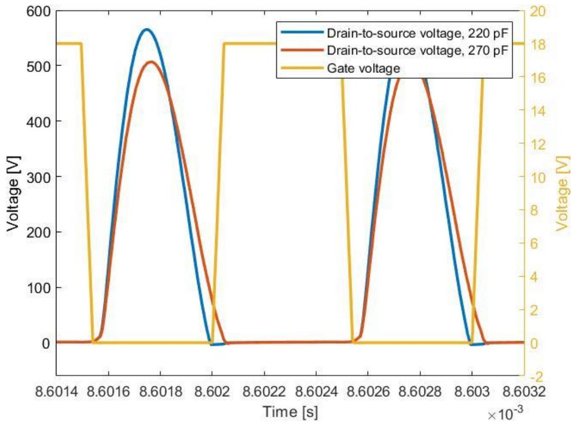
Figure 33. ZVS capability for 220 pF and 270 pF at the first suggested converter.
