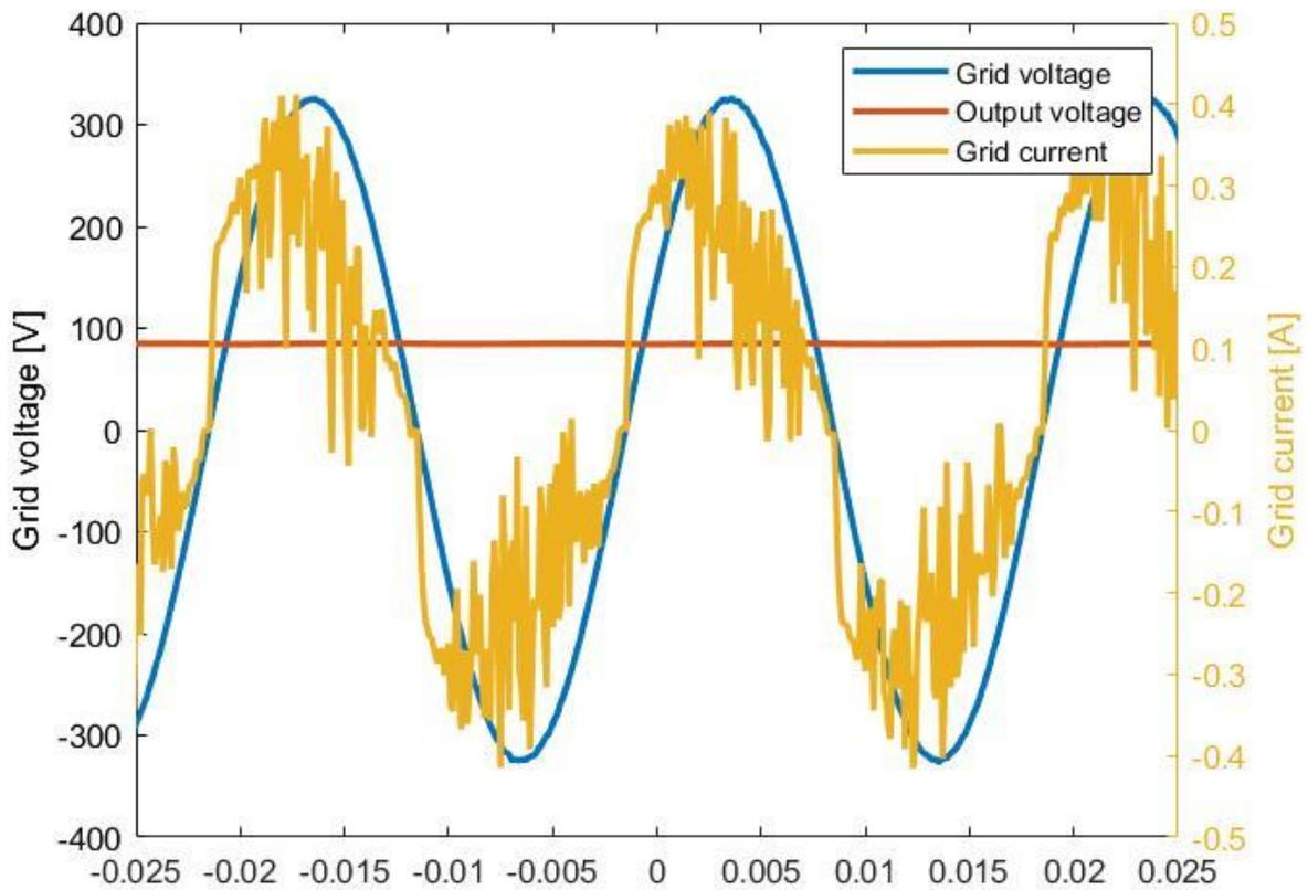
Figure 42. Grid voltage, output voltage and current across line cycle testing at 240 V/ 50 Hz for the first converter.
