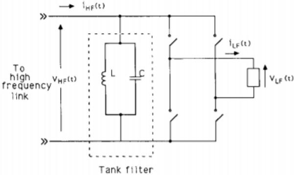
Figure 16. High-frequency link integral-half-cycle converter topology [28]
