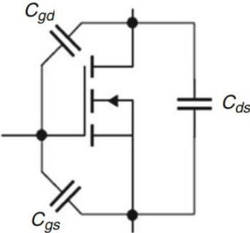
Figure 6. MOSFET with parasitic capacitance
