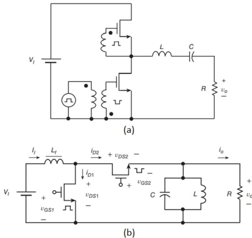
Figure 17. Class-D converter modeled as a voltage source series resonant circuit and a current source parallel resonant [20].
