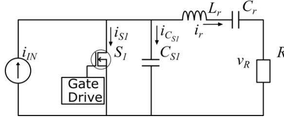
Figure 21. Class-E current source equivalent. [14], [20]
