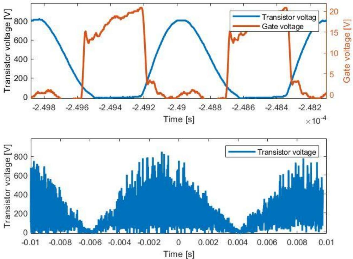
Figure 60. Drain-to-source and gate voltage across switching cycles and drain-to-source voltage across line cycle for the first converter at the second test for 240 V/ 50 Hz.
