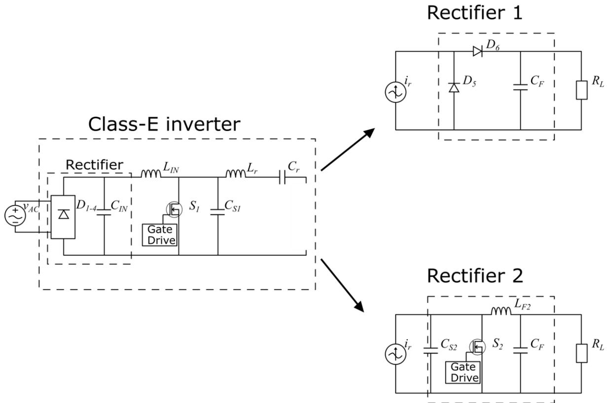
Figure 19. Class-E inverter with suggested converter 1 and 2.
