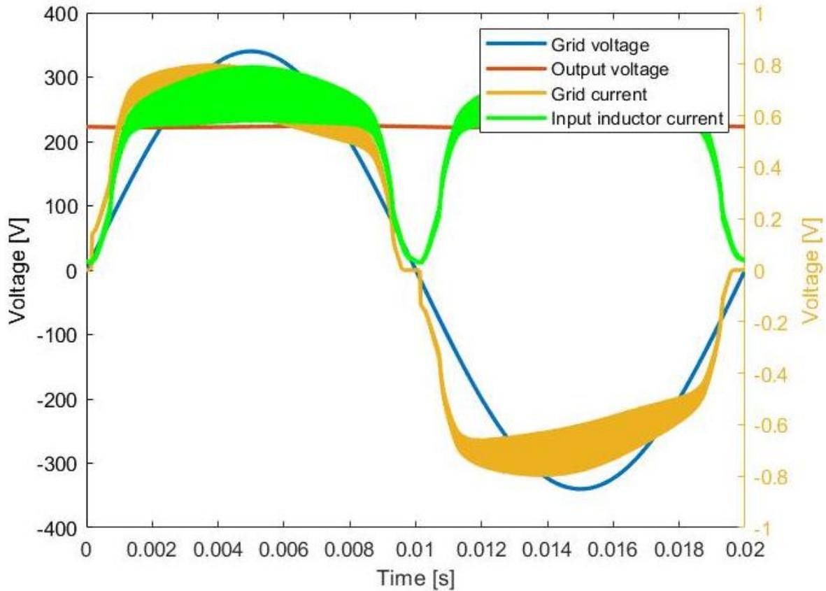
Figure 29. Simulation of grid voltage, output voltage, grid current and input inductor current of the first converter
