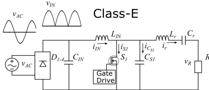
Figure 20. Class-E converter
