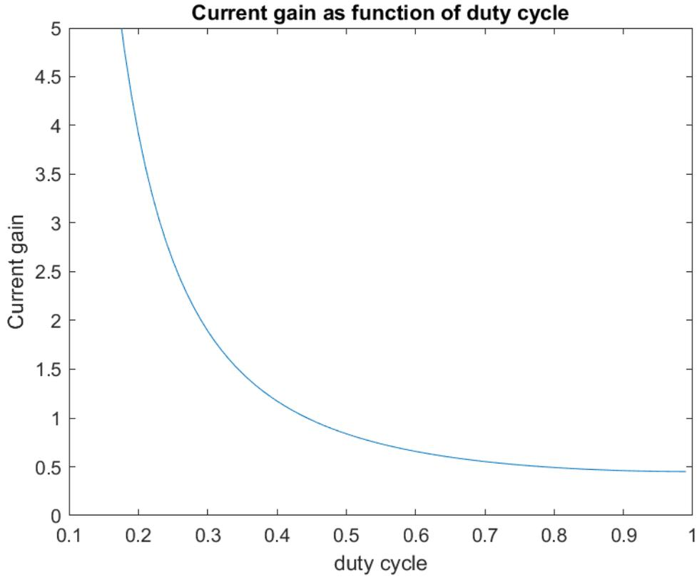
Figure 24. Current gain through the proposed converter 1.
