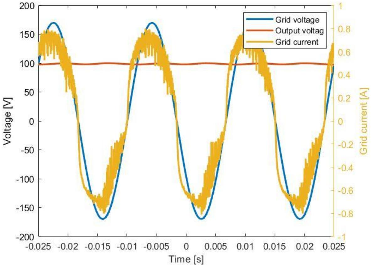
Figure 49. Grid voltage, output voltage and grid current for the second suggested converter at 120 V/ 60 Hz.
