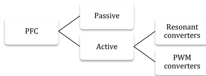
Figure 5. PFC topologies divided into active and passive circuits.
