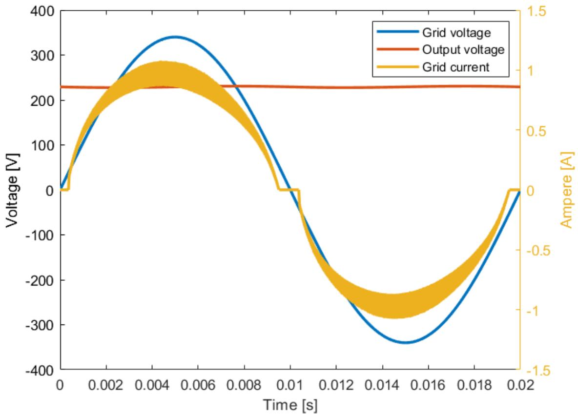
Figure 35. Simulated grid voltage, output voltage and grid current for suggested converter 2.
