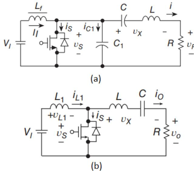
Figure 18. Class-E ZVS circuit and Class-E ZCS circuit [20].
