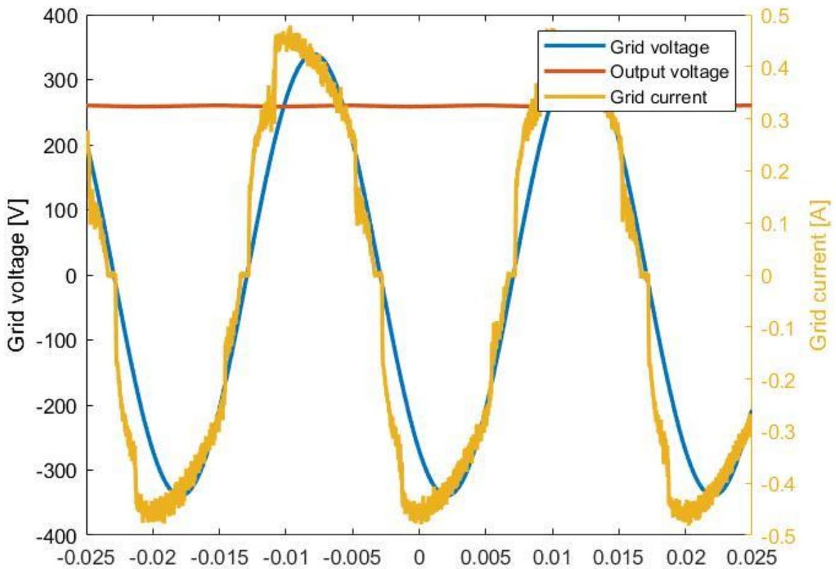
Figure 58. Grid voltage, output voltage and grid current for the first suggested converter at the second test for 240 V/ 50 Hz.
