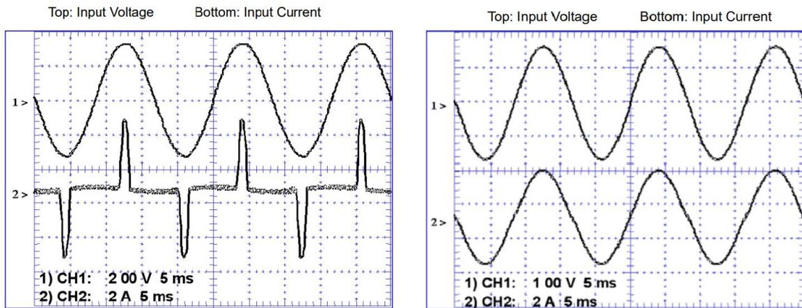
Figure 3a shows low power factor and a high amount of harmonic distortion. Figure 3b shows low harmonic and a power factor close to one [4].
