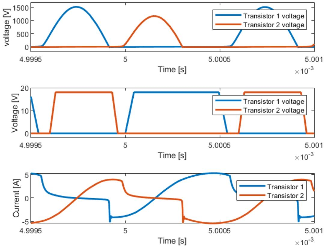
Figure 37. Simulated switching-frequency-cycle result of the transistor gate voltage, drain-to-source voltage and drain-to-source current for the second suggested converter.
