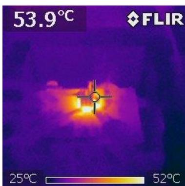
Figure 61. Temperature during the second test of the first suggested converter at 240 V/ 50Hz.
