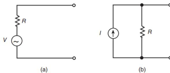
Figure 12. Voltage-source and current-source model [20].
