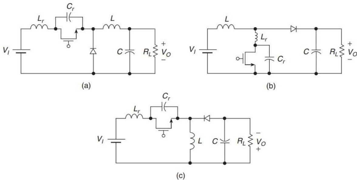
Figure 14. Quasi-resonant buck, boost and buck-boost converters: (a) Quasi-resonant buck converter. (b) Quasi-resonant Boost converter. (c) Quasi-resonant Buck-boost converter topology [6].
