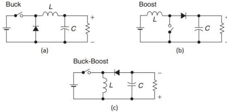
Figure 9. Buck, boost and Buck-boost converter topologies [6].
