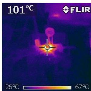
Figure 45. Temperature during testing of the first suggested converter at 240 V/ 50Hz.
