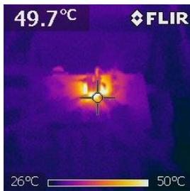
Figure 65. Temperature during the second test of the first suggested converter 120 V/ 60Hz.
