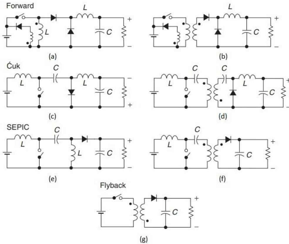
Figure 8. Different isolated and non-isolated converters [6].
