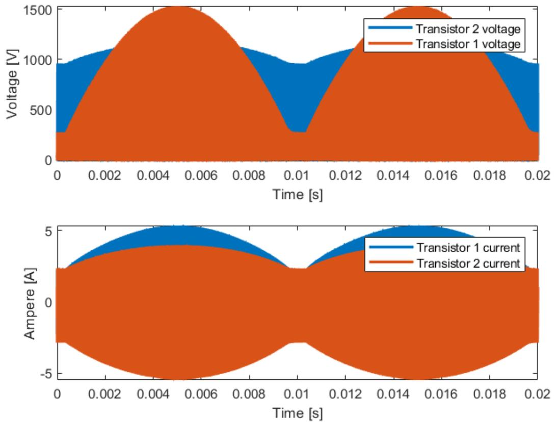
Figure 38. Simulation of drain-to-source voltage and current across one periode of 50 Hz for the second suggested converter.
