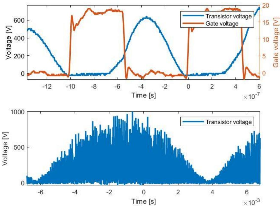
Figure 44. Drain-to-source and gate voltage across switching cycles and drain-to-source voltage across line cycle for the first converter.
