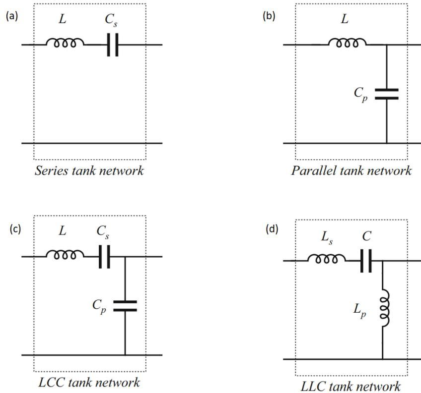
Figure 13. Series resonant tank, parallel resonant tank and hybrid resonant tank [19].
