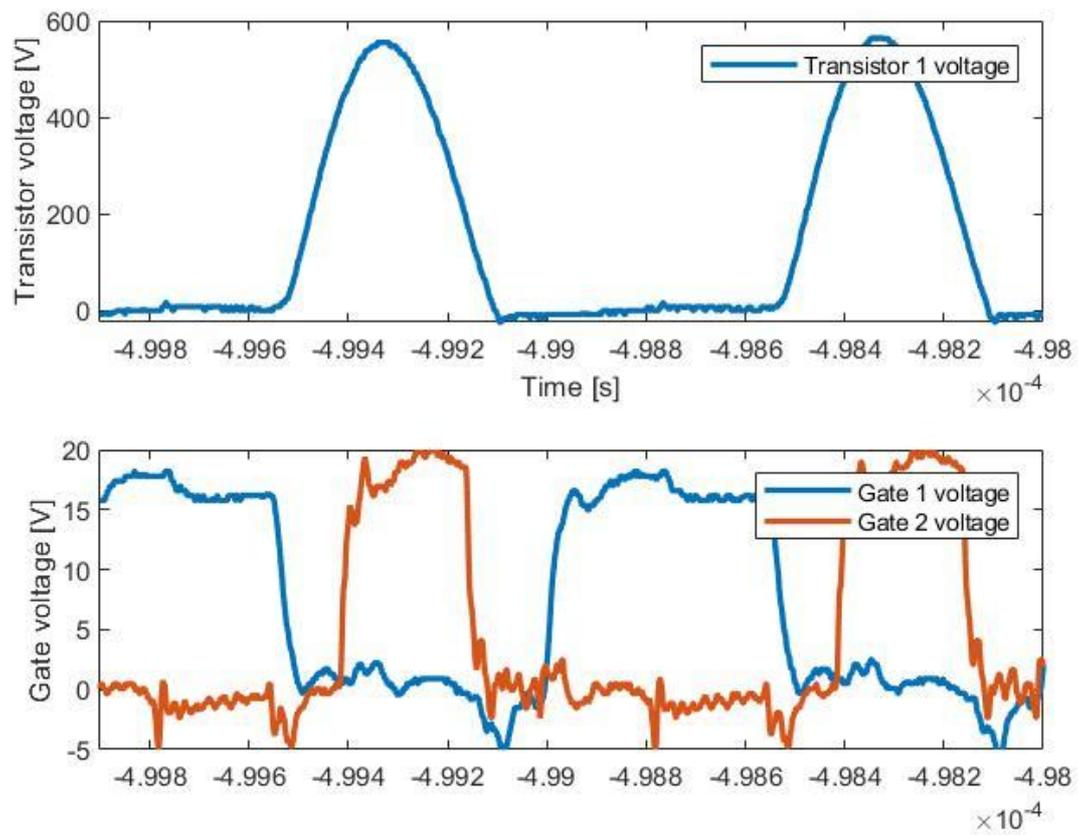
Figure 51. Drain-to-source voltage of transistor 1 and gate voltage of transistor 1 and 2 for the second suggested converter at 120 V/ 60 Hz.
