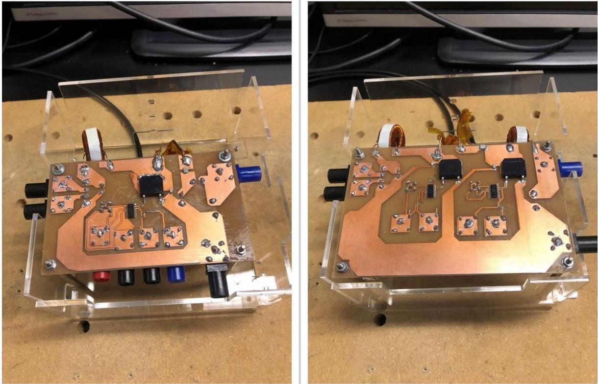
Figure 27. The first and second suggested converter designed at UiT campus Narvik.
