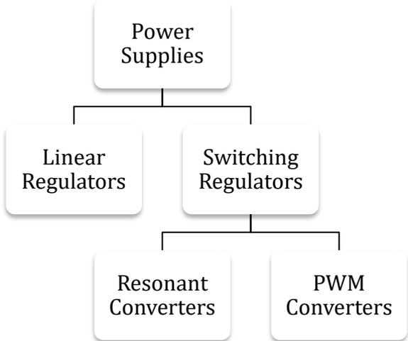
Figure 4. Power supplies divided into Linear Regulators and Switching Regulators.
