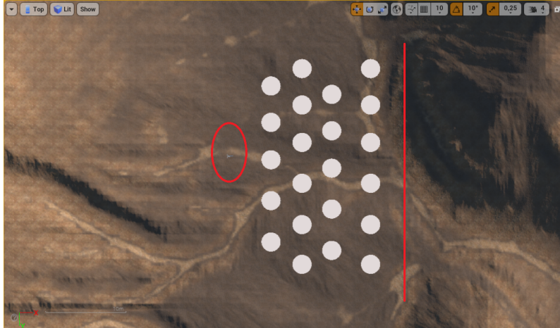
Figure 12: Top-down view of scene setup with barriers (white circles), starting are of the swarm (red circle), and finish line (red line)
