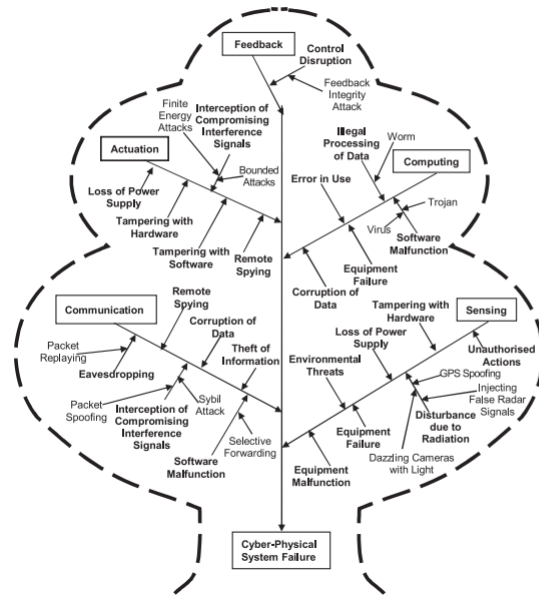
Figure 2.9: A tree diagram of attacks and threats on cyber-physical systems, adapted from [20]
