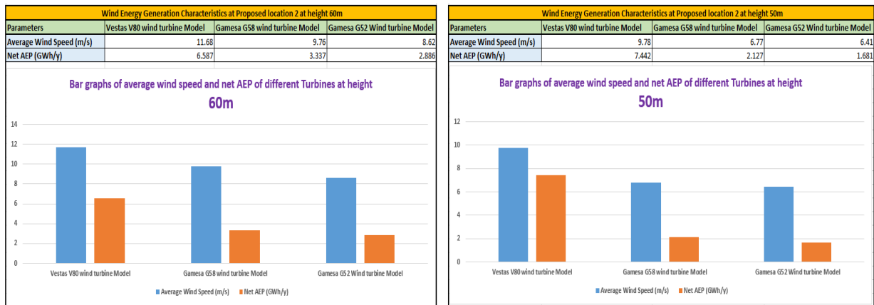
Figure 4-31: Comparison of different wind turbine model performance at hub height 50m (right) and 60m (left) virtually sited at the proposed location of choice.
