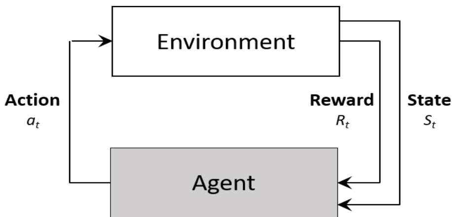
Figure 3.1: The basic components of a RL system.
