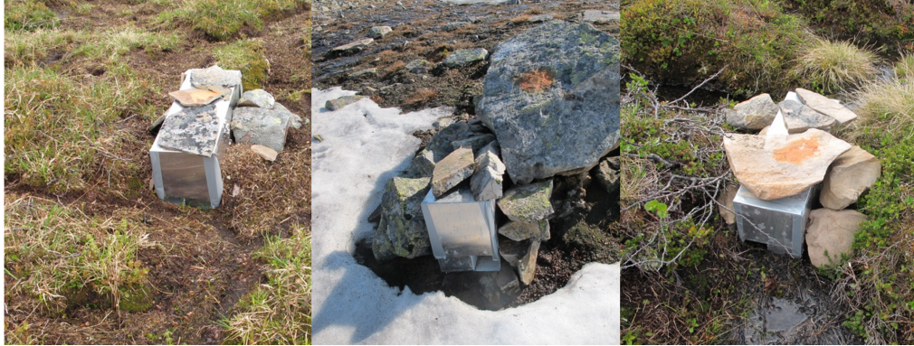
Fig. 3. Typical camera trap placements in different habitats and relations to micro-topographic features. Mesic hummock tundra with paths and grazing signs of rodents (left panel). Snow bed in early July (centre panel). Hummock tundra where the camera was damaged by flooding during the spring thaw (right panel).
