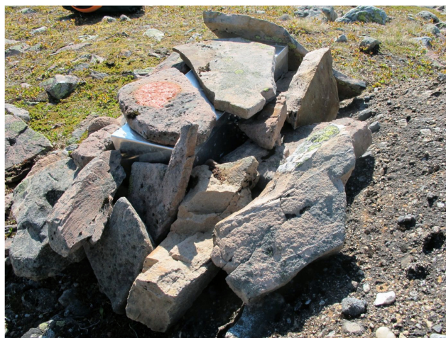
Fig. A2. Example of a camera trap embedded in a stone pile made to prevent infiltration of drifting snow that may clog the trap as shown in Fig. A1, Snow 3.
