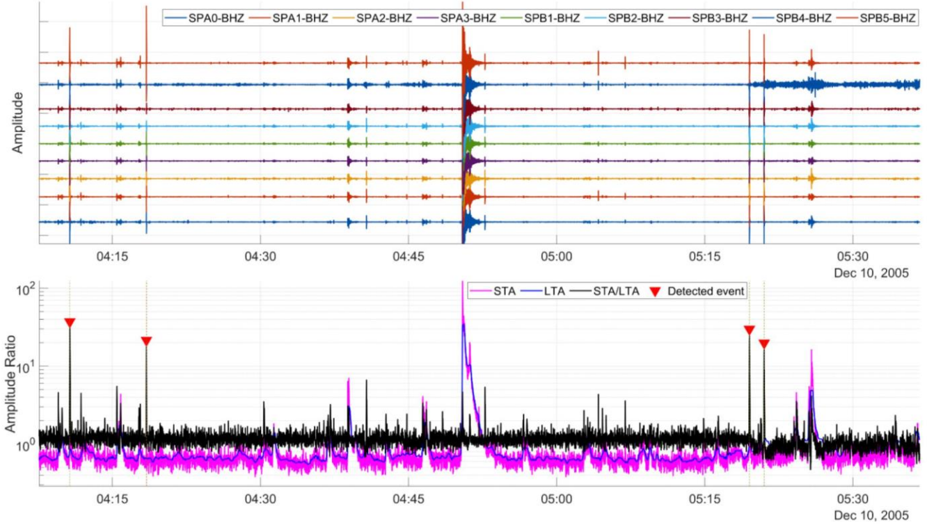
155 Figure 3 – Example of event detection using the STA/LTA (short term/long term average) detector. Short duration events with sufficient amplitude and array coherence are selected while longer events such as the high amplitude example at 04:50 are ignored.
