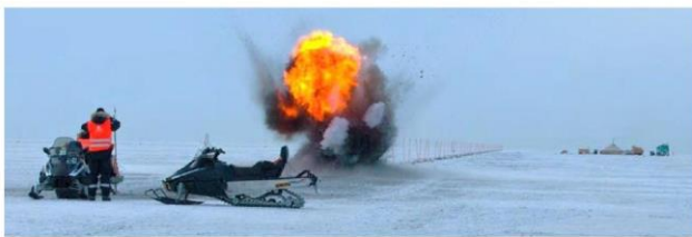
Figure 2. Photo taken during the 2013 field campaign showing the explosive seismic source. The line of seismic receivers is marked with red poles (photo: Robert Pfau).
