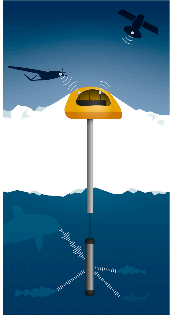
Fig. 2. An example of an ice-tethered observatory. This example is of the bio-acoustic observatory.
