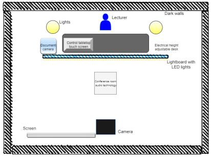
Fig. 4. A scheme of a planned Lightboard studio
