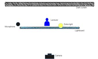
Fig. 1. A scheme of the first prototype of a Lightboard studio, <u>https://app.diagrams.net/</u>
