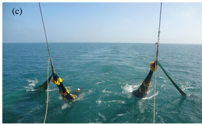
Fig. 2. Schematic view of the fishing gear configuration tested in the experiments. (a): the fishing vessel and specification of the tested codends, (b): the vessel towing two trawls simultaneously, and (c): the haul-back process of the tested codends.
