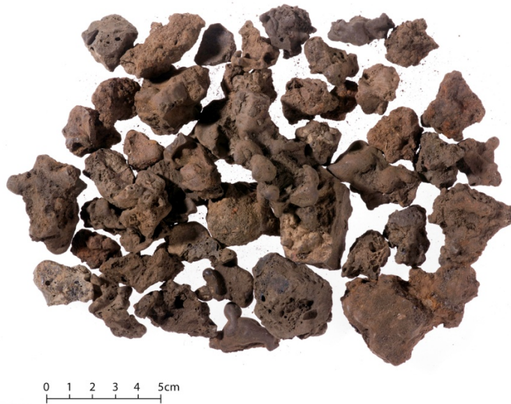
Figure 22 - Slag found next to the furnaces (Photo: Adnan Icagic, Tromsø University Museum)
