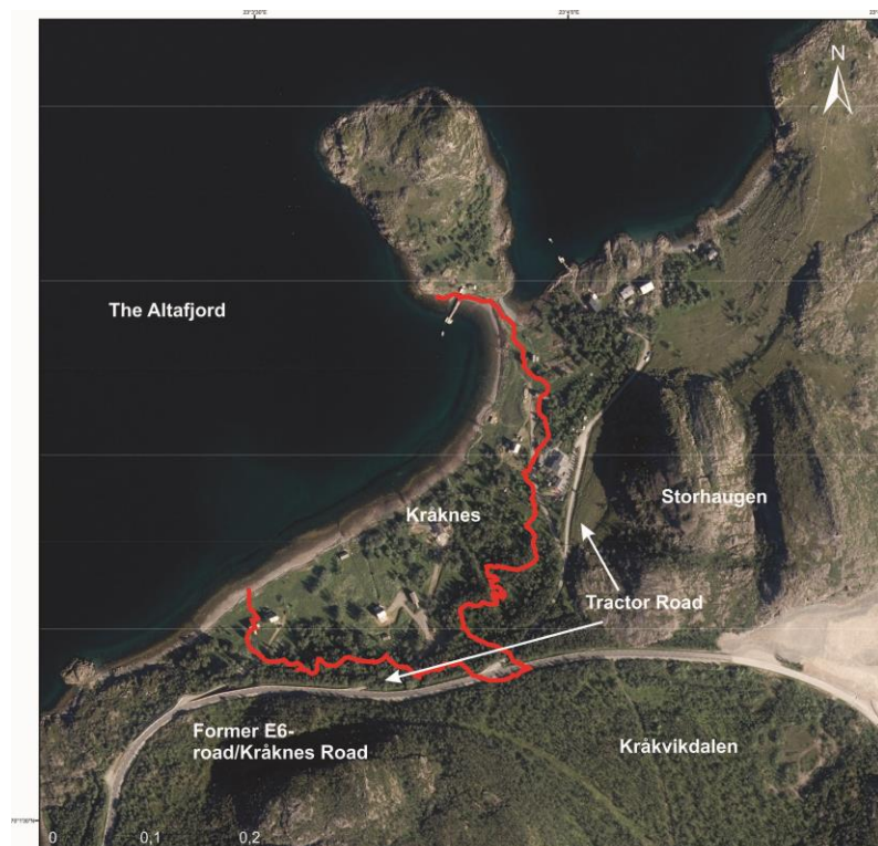
Figure 37 The study area described in this section. The red line is the back scarp.
