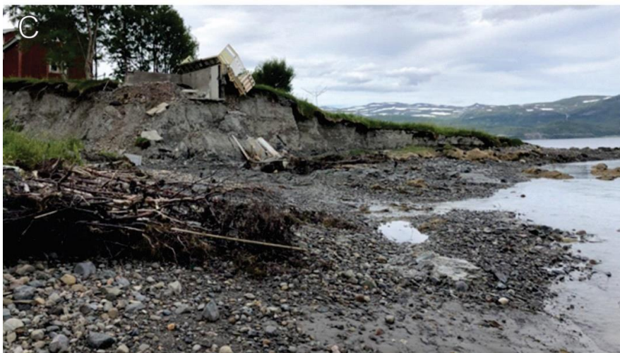
Figure 43 A) Outcrop 1 in section A with bedding of Material 2 and 1. B) Bedding of Material 2. Inset: Material 1 when remolded between fingers. C) Material 1 surface exposed during low tides.
