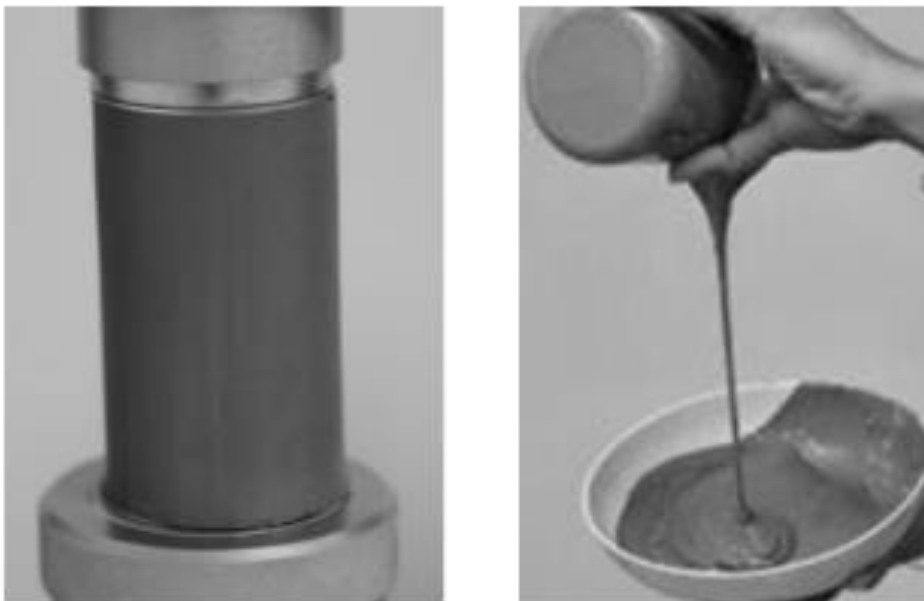
Figure 18 Highly sensitive clay in intact condition (left) and in fully remoulded state (right) (Thakur & Nigussie, 2014).
