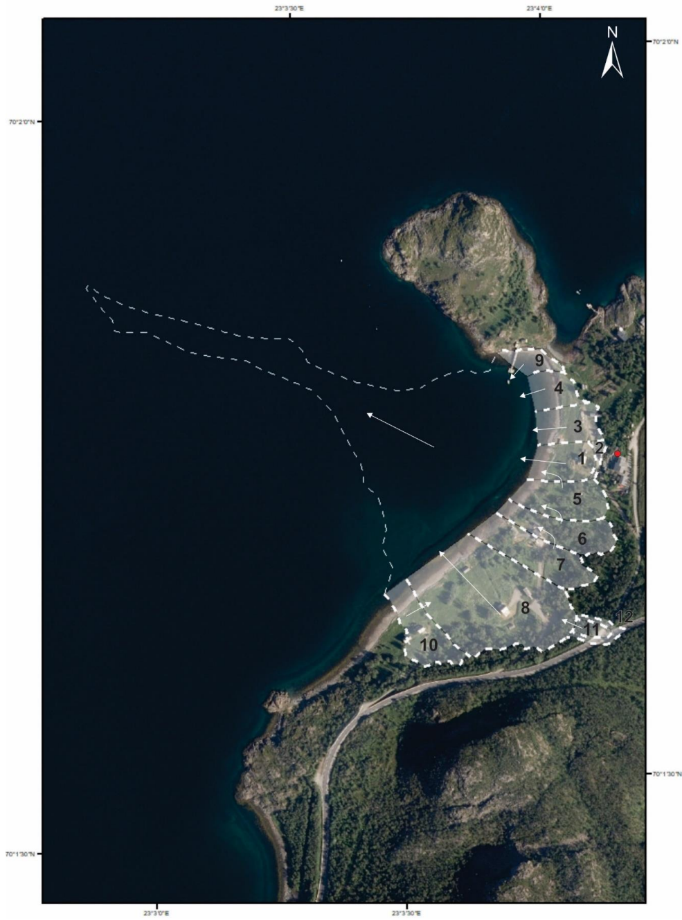
Figure 74 Map of the sequence of the landslide event. The numbers indicate in what order the area slid out. The red circle is the location of the eyewitness on who this reconstruction map is based on. Arrows show sliding direction (Based on the information provided by Anders Bjordal from NVE during fieldwork).
