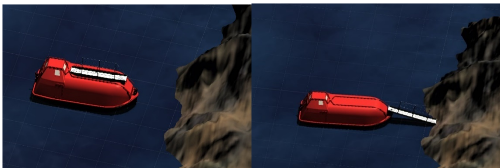
Figure 12: (a) To the left, sliding gangway. (b) To the right, sliding gangway deployed
