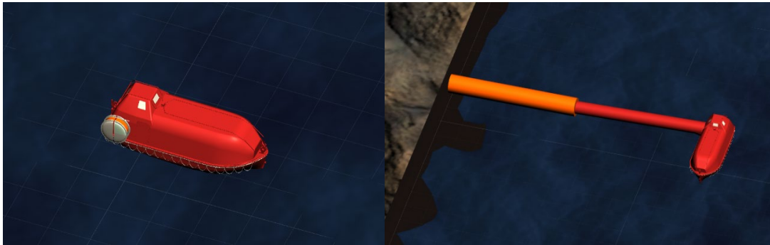
Figure 15: (a) To the left, tube casing attached to the lifeboat. (b) To the right, deployed tube gangway.
