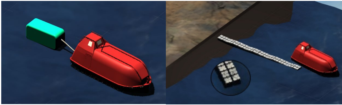
Figure 13: (a) To the left, enclosed floats attached to the lifeboat. (b) To the right, deployed fastened floats.
