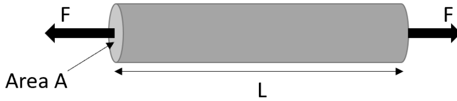
Figure 25: A cable with forces acting in both directions.
