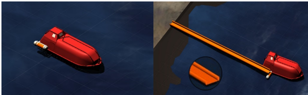
Figure 14: (a) To the left, attached inflatable gangway. (b) To the right, deployed inflatable gangway.
