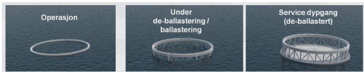
Figure 29: NRS AOF cage, under operation (semi submerged), under ballasting and de-ballasted for servicing: Image modified from Arctic Offshore Farming (2021)
