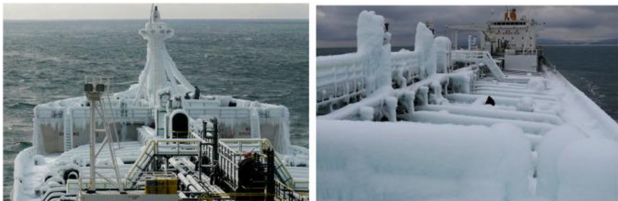
Figure 11: Sea spray icing on vessel. Modified from Group Ocean (2010)
