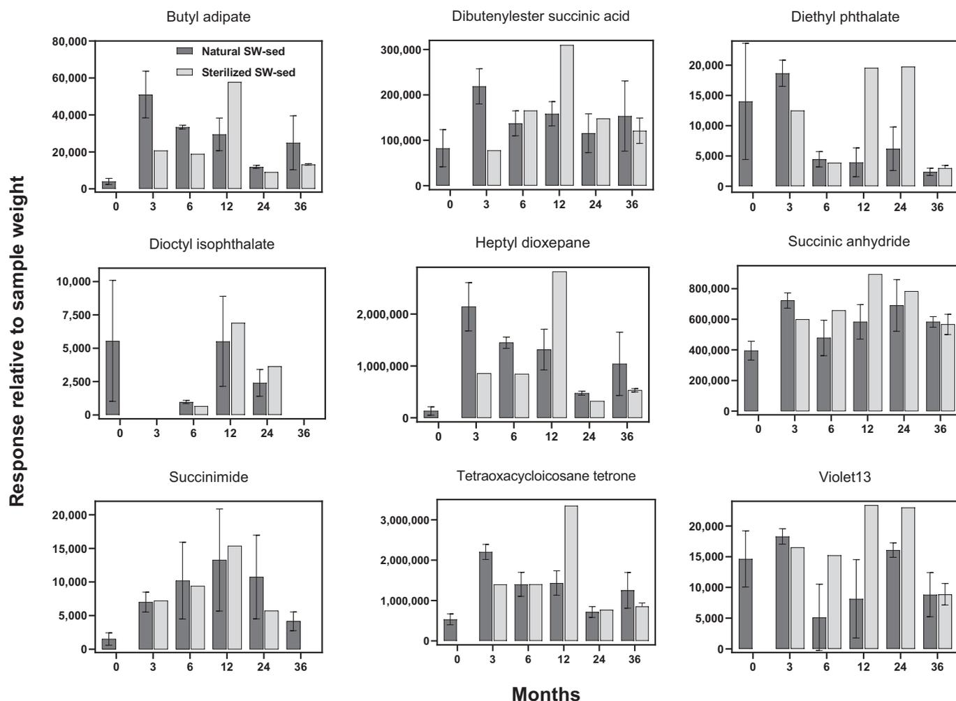
Fig. 6. Relative responses of compounds potentially identified by thermal desorption GC/MS analyses of PBSAT filaments in biotic and sterilized SW-sediment (0–36 months). The error bars represent standard deviations from measurements of 3 replicates.
