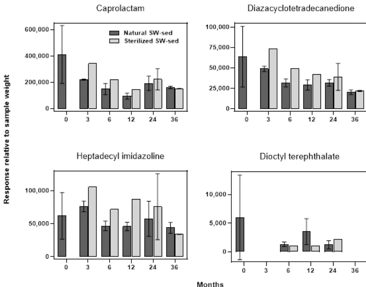
Fig. 5. Relative responses of compounds potentially identified by thermal desorption GC/MS analyses of nylon filaments in biotic and sterilized SW-sediment (0–36 months). The error bars represent standard deviations from measurements of 3 replicates.
