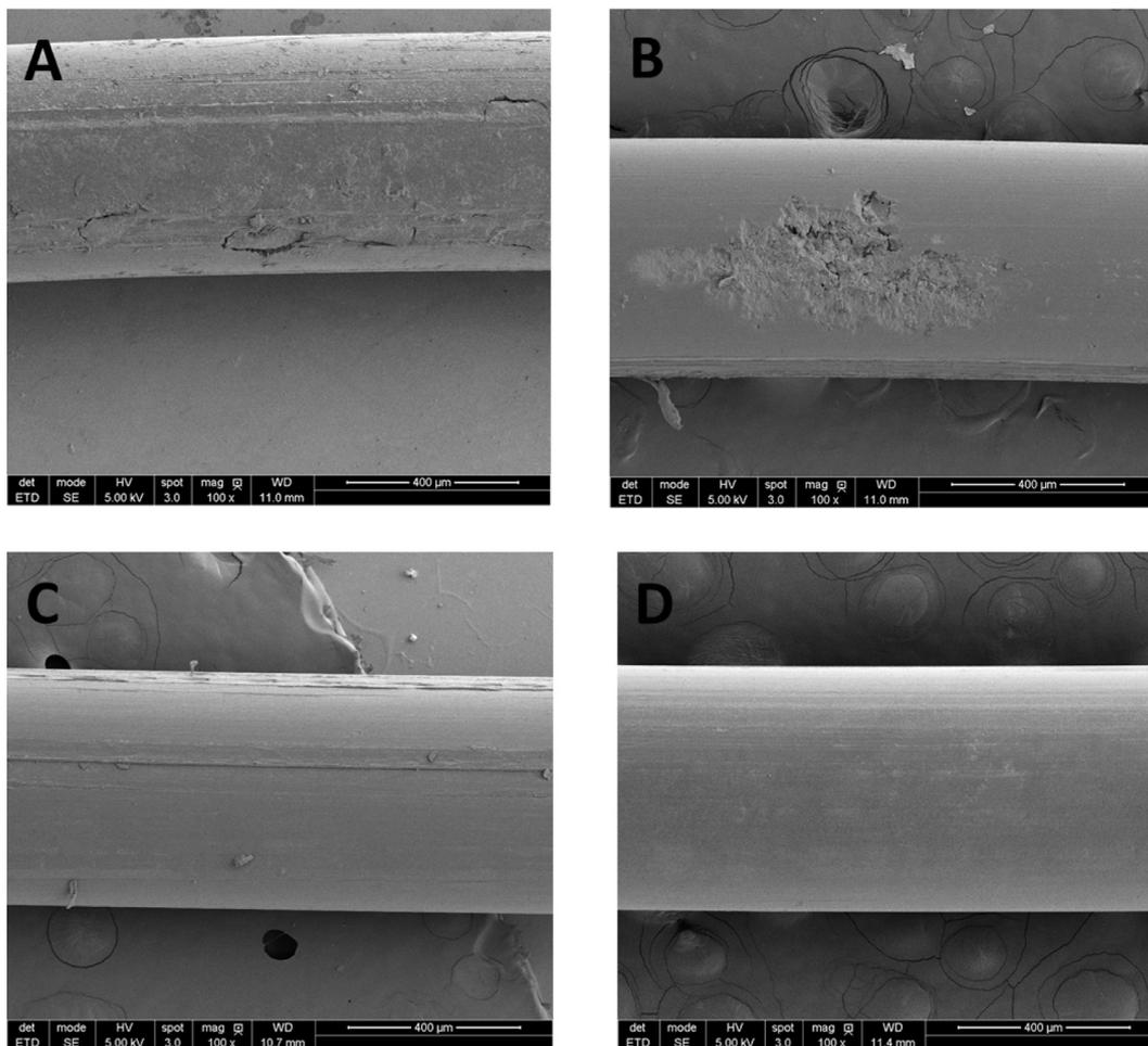
**Fig. 1.** SEM analyses of PBSAT (A–C) and nylon (D) gillnets after 36 months of incubation in SW-sediment systems. The nets were incubated in static systems with normal (A, B and D) or sterilized SW (C).
