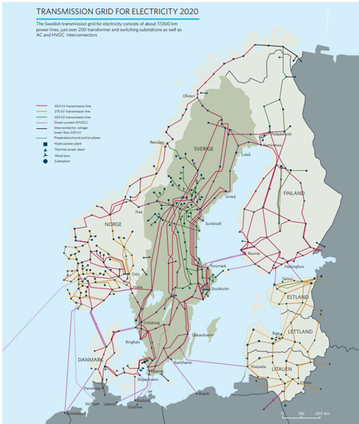
Figure 7: Overview over transmission lines in the Nordic and Baltic countries. The red lines indicate 400 kv, the orange lines 275 kv and the green lines 220 kv transmission lines. The transmission lines have not capacity to transmit all of the surplus energy from the northern regions (NO4 and SE1) and southwards. This result in price differences in the Nordic electricity market [69].
