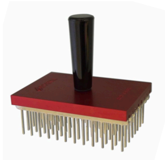
Figure 3: 96-replicator pin (Boekel Scientific)
