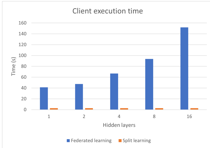
Figure 6.1: Raw execution time to perform each methods training on the client for 50 epochs
