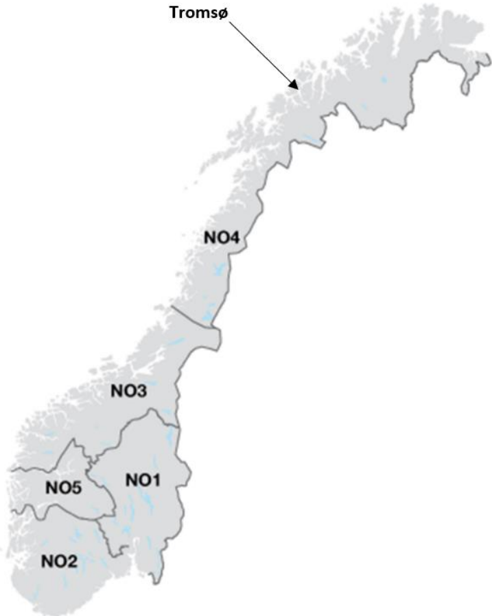
Figure 13: The five price regions in Norway, made due to limitations in transmission capacity. Tromsø is in price region 4 (NO4) (Statnett, 2022).
