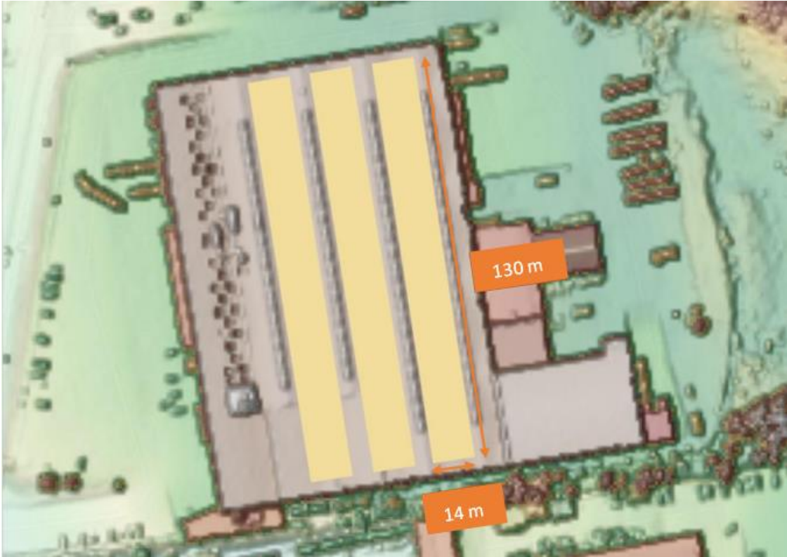
Figure 16: Assigned area for module installation on Coops warehouse roof, consisting of three similar columns with individual dimensions of 14 m* 130 m, forming a combined area of 5460 m 2 .
