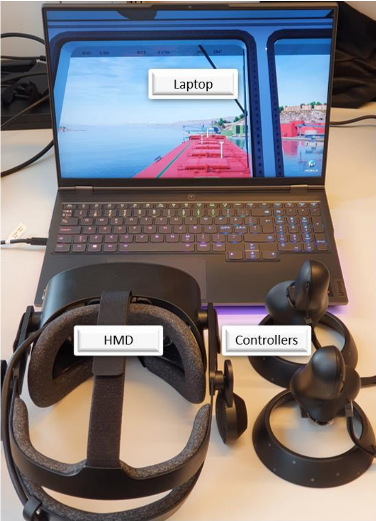
Figure 4 - Morild VR simulator setup with HMD, controllers, and laptop.
