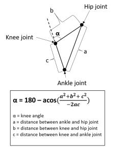
**Figure 2**. The knee angle measurement procedure of the CV prototype
