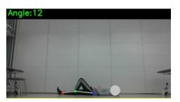
**Figure 4.** Example where the CV prototype confuses the knee joint of the left leg with the right leg and hence provides an erroneous measurement result
