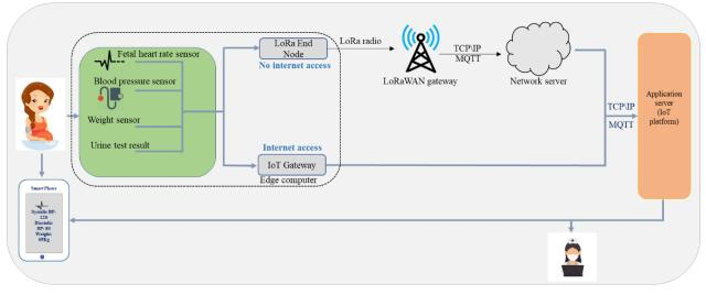
Figure 1. Schematic diagram of the proposed architecture.
