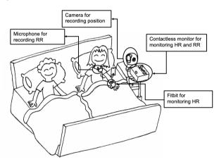
Figure 1. Illustration of experimental setup.
