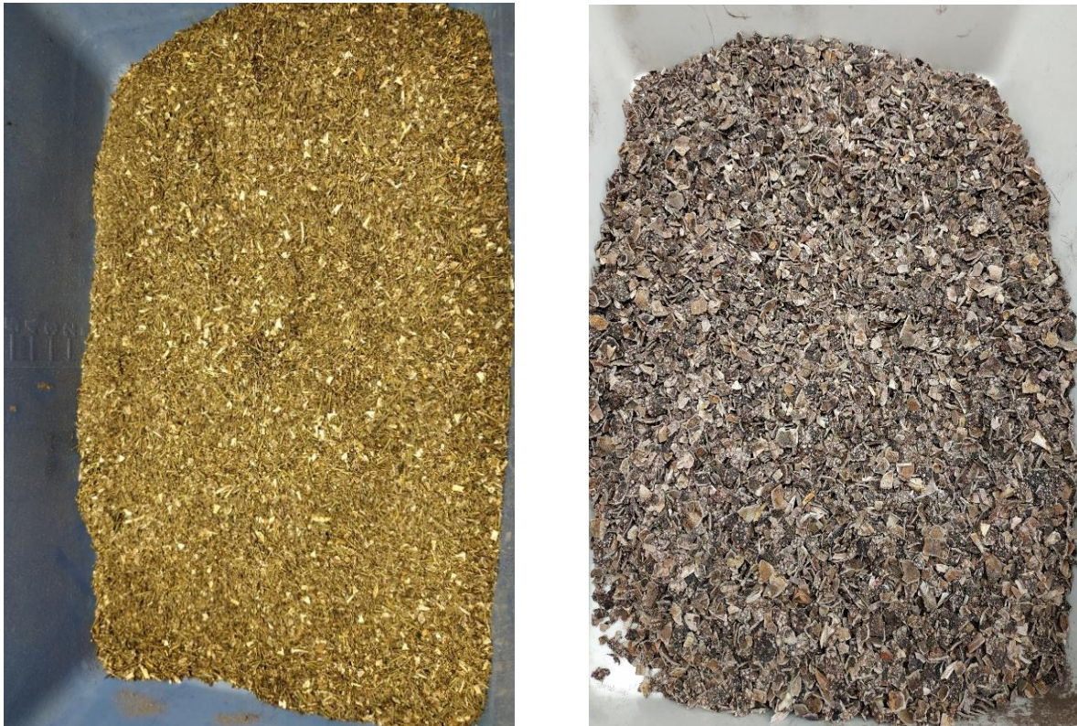
Figure 3: Sea urchins rough crush; (left) The rough crush of sea urchins relatively small and homogenous particles after being filtered through a metal sieve of mesh size 2.5 mm; (right) large and uncrushed particles that were discarded
