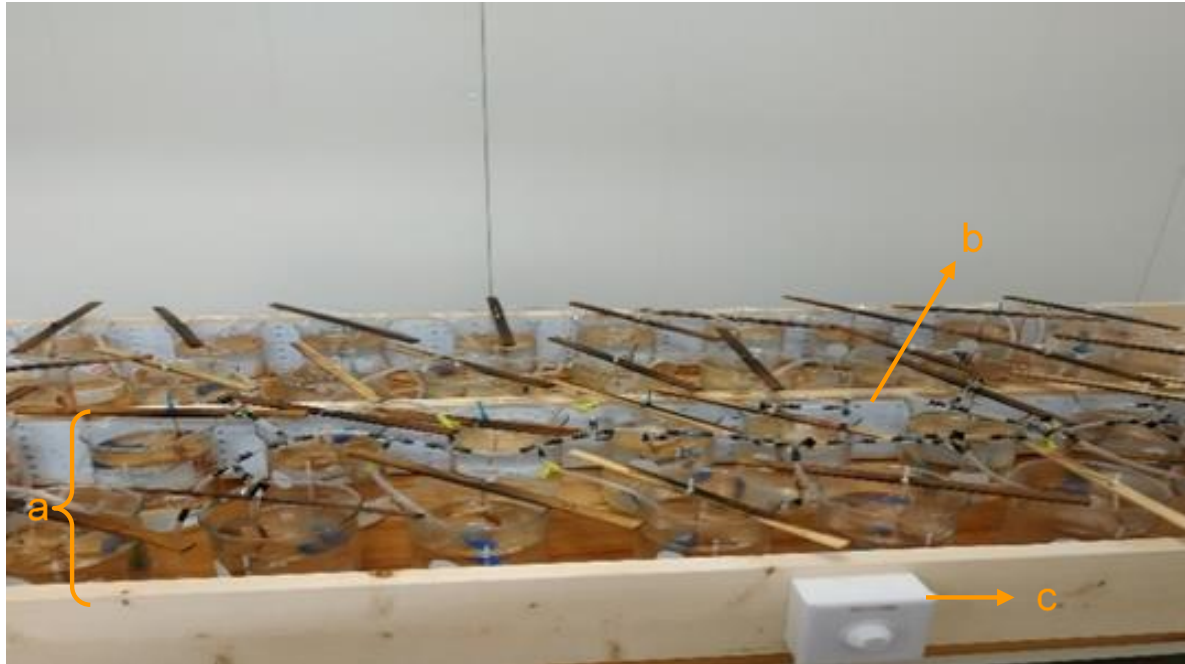
Figure 4: The experimental set-up in the laboratory in Nofima, Breivika, Tromsø with (a) two-row beakers on each side. (b) LED light is attached beside the beakers. (c) The intensity of light could be adjusted through the switch.
