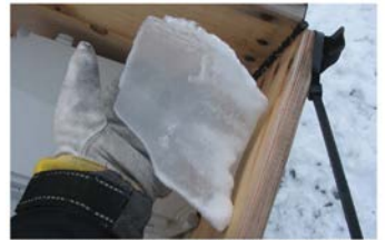
Figure 3: Piece of ice shed from a turbine in Nyglandsfjell wind park, Narvik, Norway [5]
