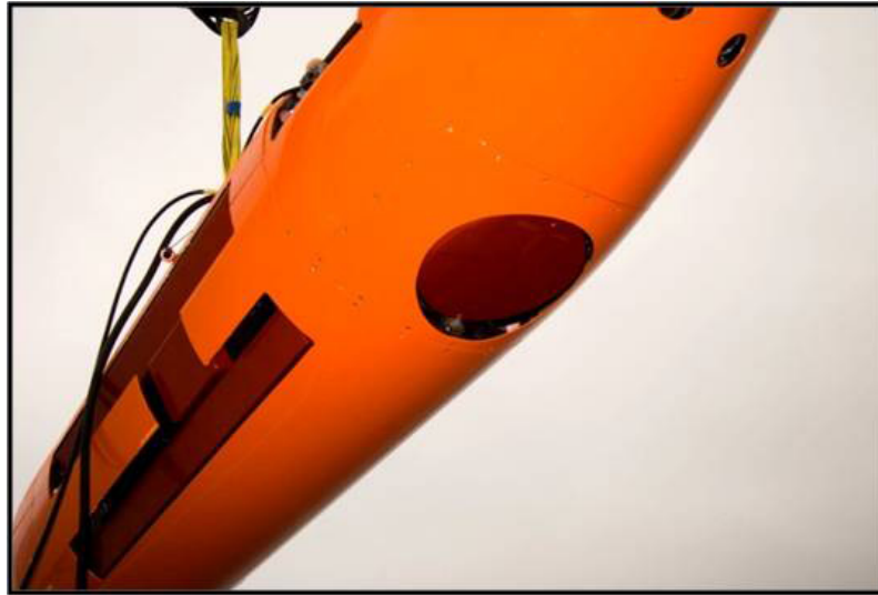
Figure 8.14: Picture of a HUGIN 1000-MR with a starboard HISAS (left part of picture) and an EM 3000.
