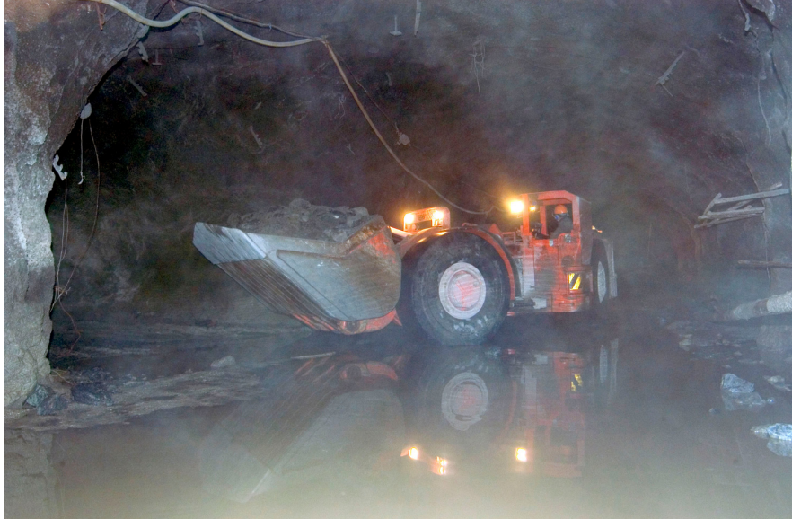
Figure 2. Toro 400 in operation in an underground mine (Photo: Arild Øvrum)
