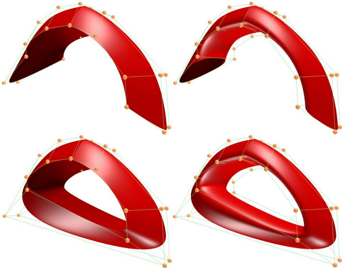
Figure 9.9: We see 4 tensor product B-spline surfaces including their control points and control polygons. The control points and polynomial degree are the same for all four. The only difference is that the upper left surface is open/clamped in both directions, the upper right is closed in one direction, the lower left is closed in the other direction and the lower right is closed in both directions.
