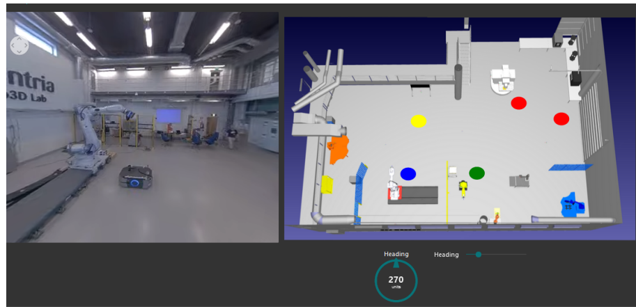
Figure 6. Control interface of mobile robot with embedded live video view.
