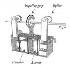
Figure 5. Powered impeller deicing device [42]
