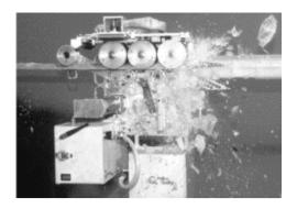
Figure 6. ROV de-icer prototype [57]
