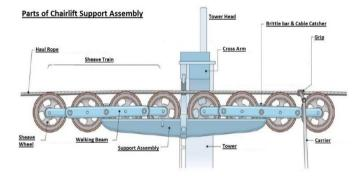
Figure 3. Gondola pillar support mechanism [23]
