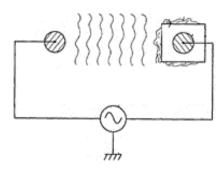
Figure 4. High frequency de-icing circuit schematics [55]
