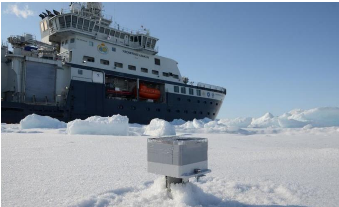
Figure 2.8.2 A sea-ice drifter frozen into the ice at the starboard side of the ship. Photo: Johannes Lohse (UiT).
