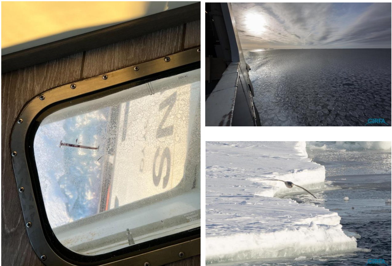
Figure 2.13.4 The left-hand image shows the downward facing window on the bridge with one metre marker, allowing the observer to estimate ice thicknesses as the ice overturns alongside the vessel. The top right image shows a fantastic example of pancake ice from deck 3 where it was easier to make the distinction as to whether the pancakes were cemented or rafter or not. The bottom right image shows how snow thicknesses were estimated after the ship had broken through the ice. There is a clear distinction between the snow layer and ice layer. All photos: William Copeland (MET).
