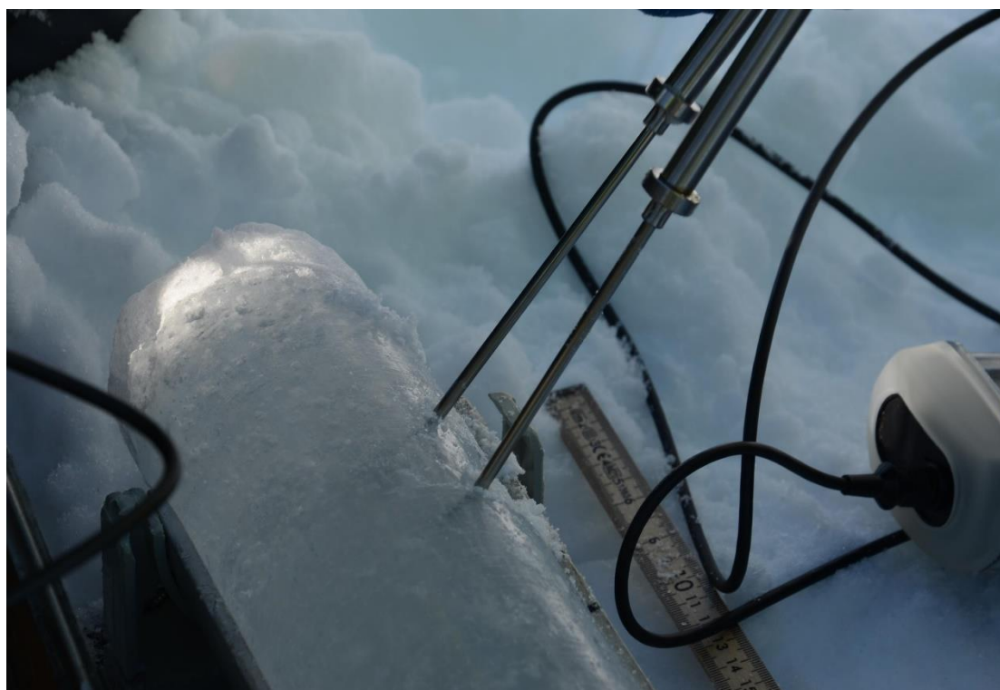
Figure 2.1.2 Temperature measurements in the field. The core is kept in the shade during processing in the field. Photo: Johannes Lohse (UiT).
