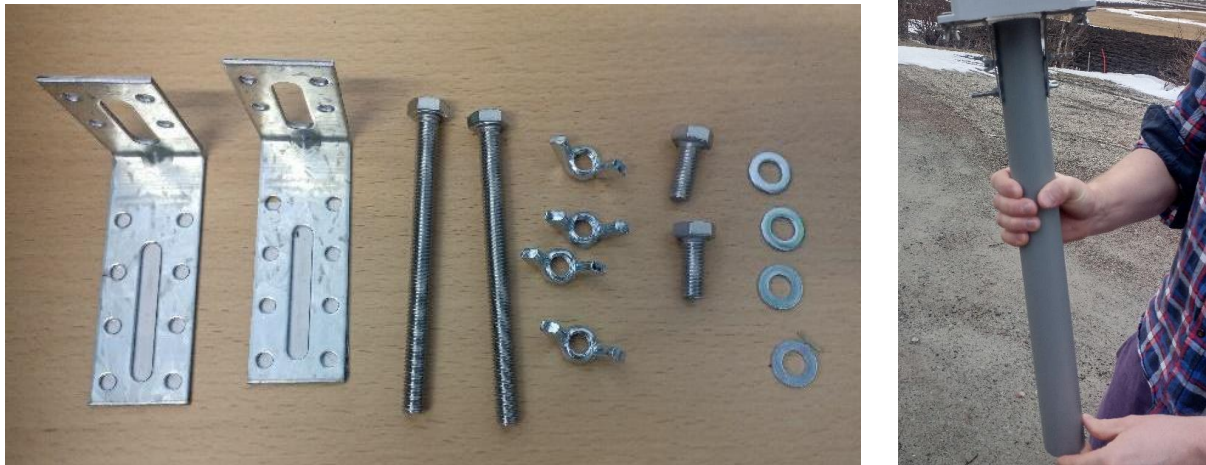
Figure 2.8.3 PVC pipe setup to freeze the drifter into the ice: materials (left) and prototype (right). Photos: Catherine Taelman (UiT).
