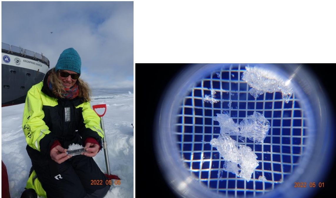
Figure 2.3.5 Left: The ice lens from CIRFA22-047 with beautiful crystals underneath (note the bottom of the ice lence is facing towards Malin). Photo: Anna Telegina (UiT). Right: Depth hoar layer crystals seen through magnifying lens. Photo: Jozef Rusin (MET).
