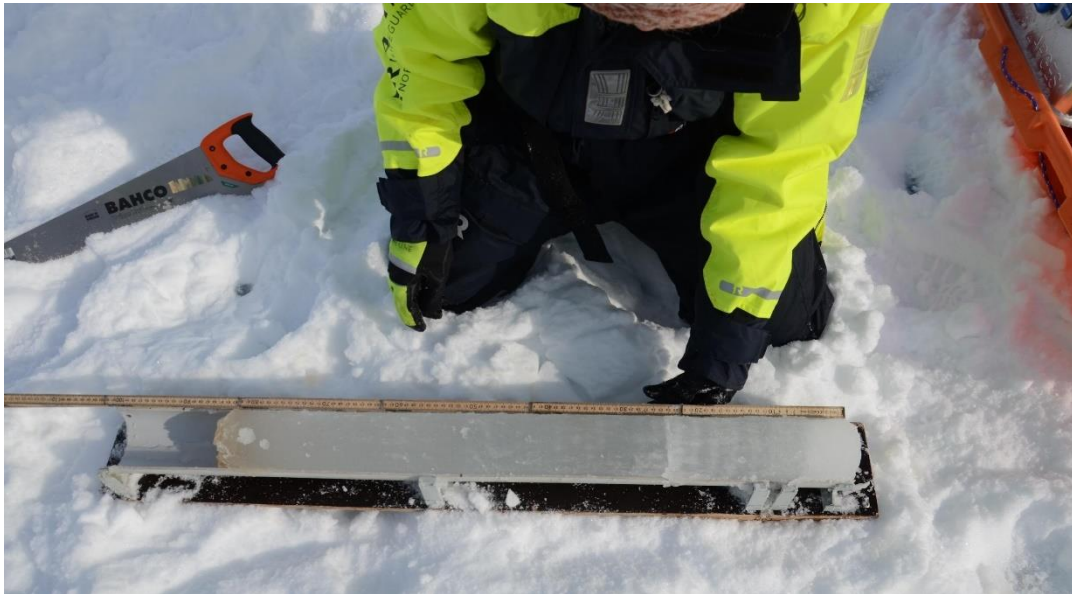
Figure 2.1.3 Ice core at Site 7 after retrieval, ready for processing. Algae are visible at the bottom (left side). Photo: Johanne Lohse (UiT).
