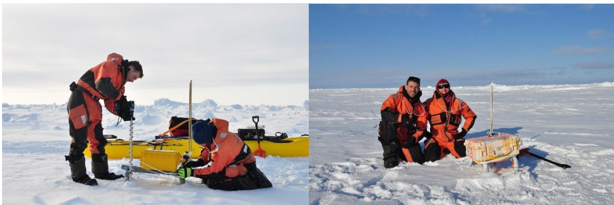
Figure 2.7.1 SIMBA deployments. (Left) drilling the 2" hole for fixing the thermistor chain in the sea ice, and (right) the final SIMBA unit sitting on a platform frozen into the ice with an air temperature sensor fixed onto a pole next to the unit. Photos: Christian Zoelly (NPI).
