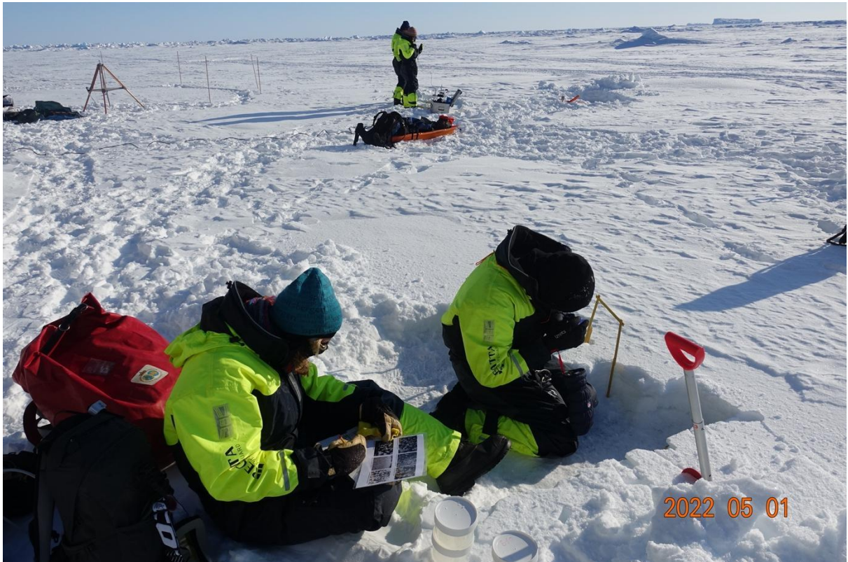
Figure 2.3.3 Snow pit from CIRFA22-034A showing Laust analysing snow grain sizes and Malin taking notes. Photo: Jozef Rusin (MET).
