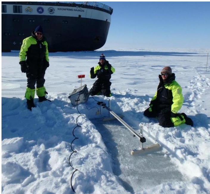
Figure 2.2.2 The surface roughness team measuring a profile over sea ice exposed with a shovel and brush. Photo: Andrea Schneider (UiT).
