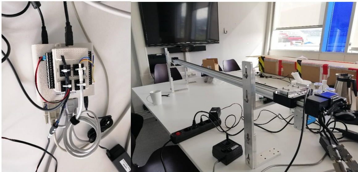
Figure 2.2.1 The roughness profiler set up in the office, showing the control box on the left and the profiling frame on the right. Photos: Anca Cristea (NPI).
