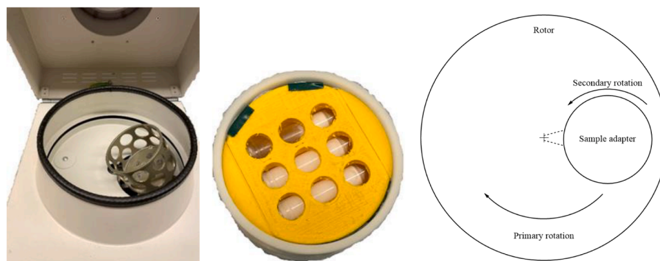
Fig. 1. Inside of the SpeedMixer™ type “DAC 150.1 FVZ-K” (left), sample adapter for 6 Twist-Top vials (middle), and schematic representation of rotation pattern (right).
