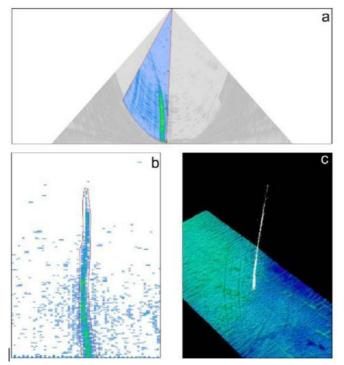
Figure 2: Gas flare cropping workflow. a - limiting the beam span to a size of a flare. b - outlining flare contours and exporting the content of the selected volume in \*.ascii format. c - importing the flare volumes to QPS Fledermaus, Petrel, etc. software.
