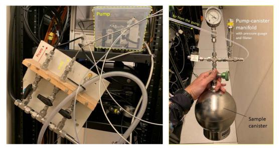
Figure 10: Equipment used for discrete air sampling via the inlet installed on the ship's mast.
