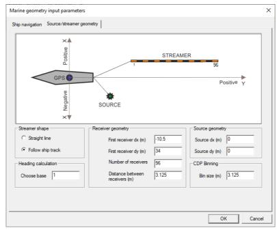
*Figure 3: Geometry of the 2D seismic survey. The gun position is used as a reference point for streamer geometry calculation.*
