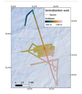
*Figure 21: Seismic and multibeam surveying over the western Sentralbanken region, east of and adjacent to the Hopendjupet Seepage Area.*
