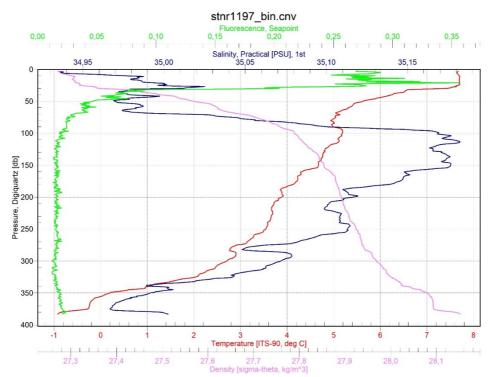
*Figure 6: An example of the salinity, temperature, density and fluorescence profiles acquired with the SBE 911 plus CTD at station 1197.*
