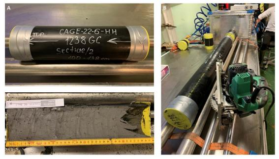
Figure 8: Sediment core processing. A – core liner cut in sections; sections are labelled and sealed. B – core liner ready for splitting with a rotary saw. C – split open core section ready for subsampling and description.
