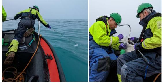
*Figure 9: Sampling oil slicks from the working boat using a ETFE membrane at station 1248 (Photos: H. Patton).*
