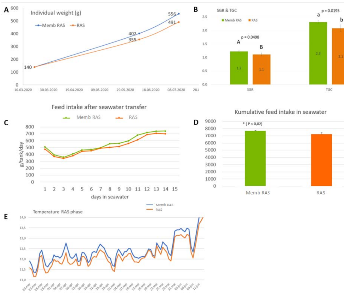
Figure 4 A) Weight development during the experiment (g). B) SGR and TGC values for the whole experiment. C) Feed intake after seawater transfer D) Cumulative feed intake in seawater E) Temperature in the RAS phase. N=4 tanks per treatment. MembRAS indicates RAS with nanofiltration membrane and RAS is the control system without nanofiltration.
