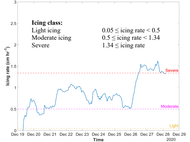
FIGURE 4: ICING RATE DURING VOYAGE OF ONEGA ACCORDING TO MINCOG OPERATIONAL VERSION
