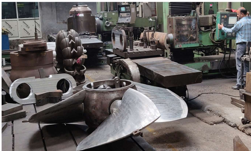
Figure 19 An impeller with separate blades (Source: Metrology News)
