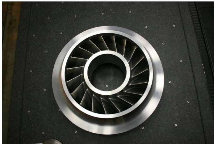
Figure 21 One-piece machined impeller (Source: Metalex)
