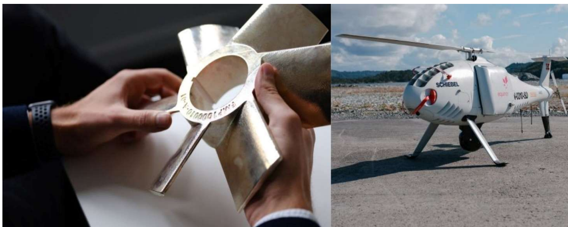
Figure 3 3D printed part (L) and drone used to transport the printed part (R) (Source: Equinor)
