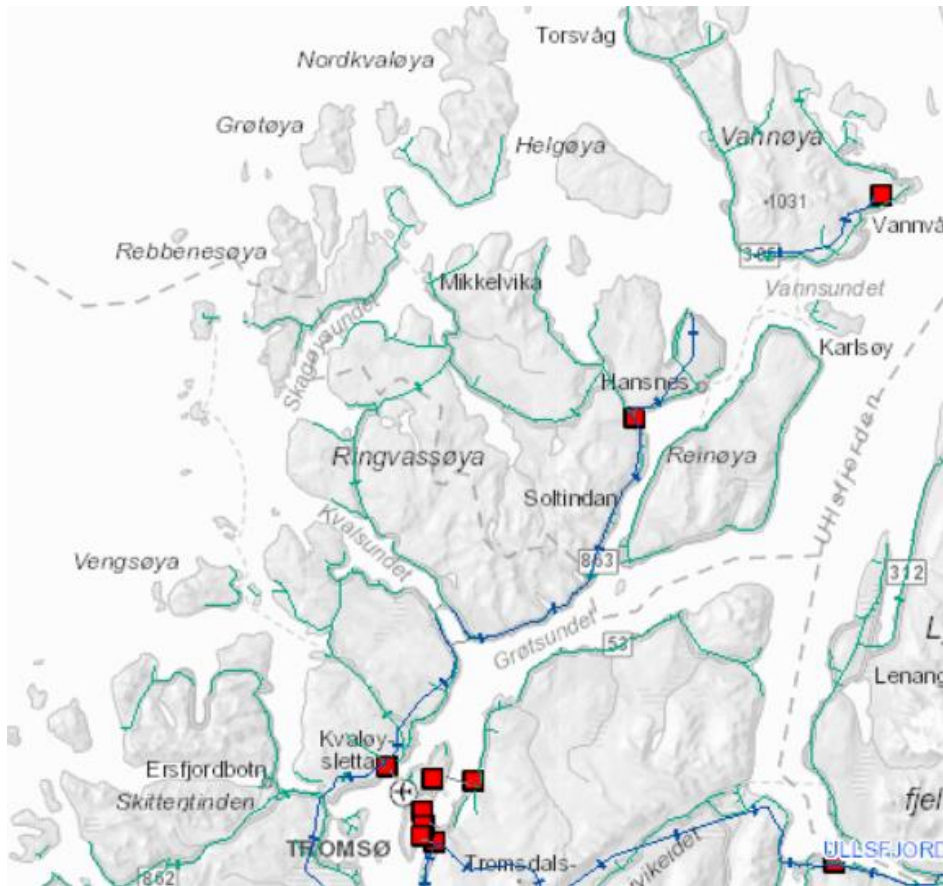
Figure 18: Parts of transmission grid north of Tromsø.
