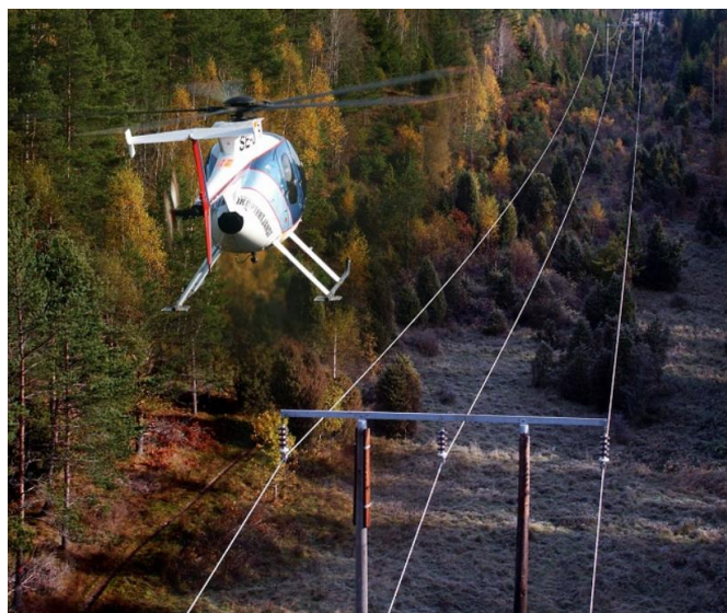
Figure 15: Power line inspection using helicopter
