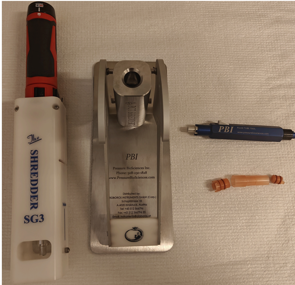
Figure 10. From the left, SG3 Shredder, PBI shredder base, PBI tube tool, and shredder tube with two lids. Oroboros Auxiliary HRFR-Tools (Draxl et al.)
