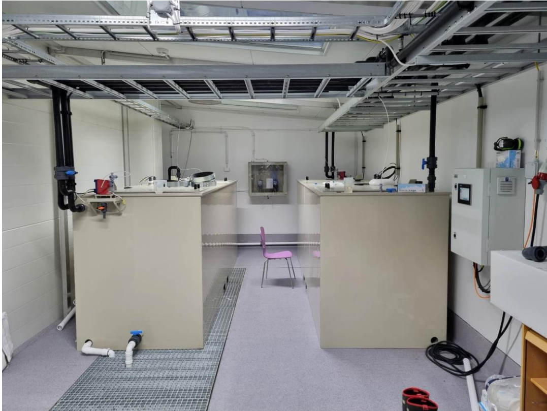
Figure 8 Both maturation tanks used in the experiment. The left maturation tank in the picture had inoculum added, while the right one is control.
