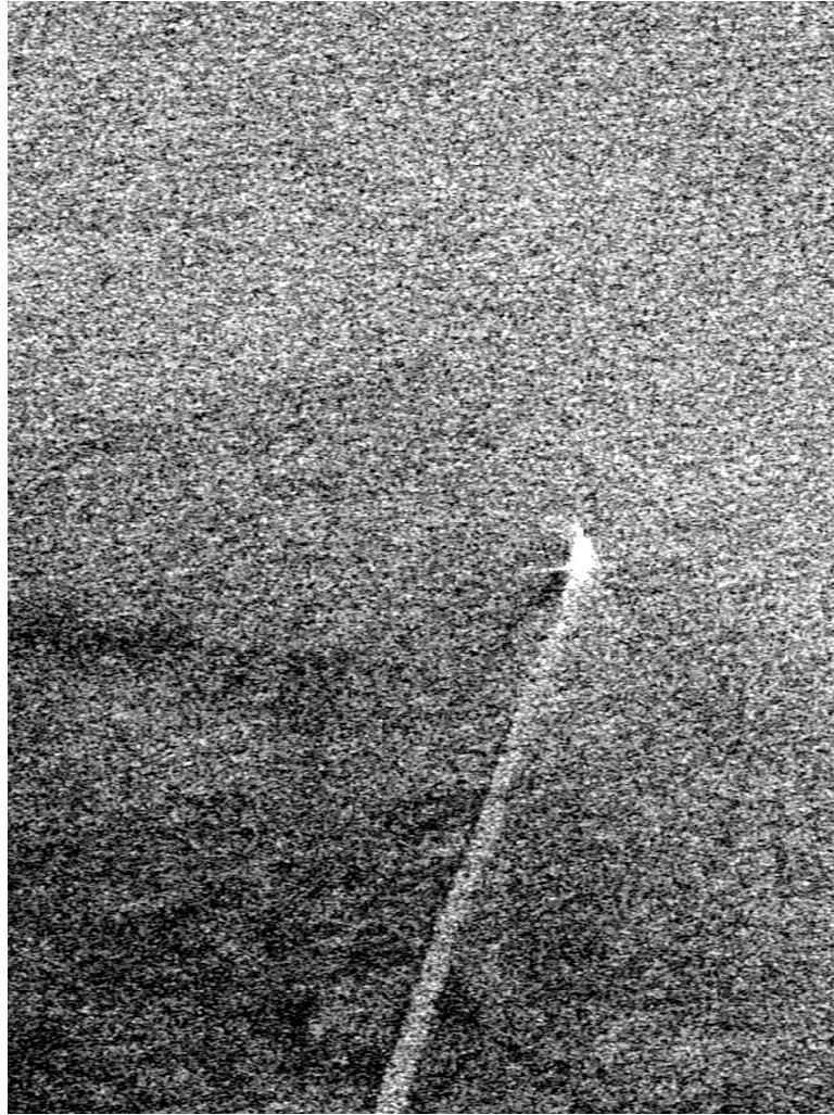
Figure 2.5: A Sentinel-1A image from 2020-04-18 calibrated to Sigma zero. The bright spot is a vessel with a wake. The brighter tail behind is the turbulent wake as the ship moves through a low wind ocean.
