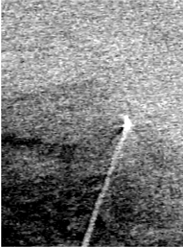
Figure 2.6: A Sentinel-1A image from 2020-04-18 calibrated to Sigma zero with a 5x5 multi-looked window. The image is the same as seen in Figure 2.5.
