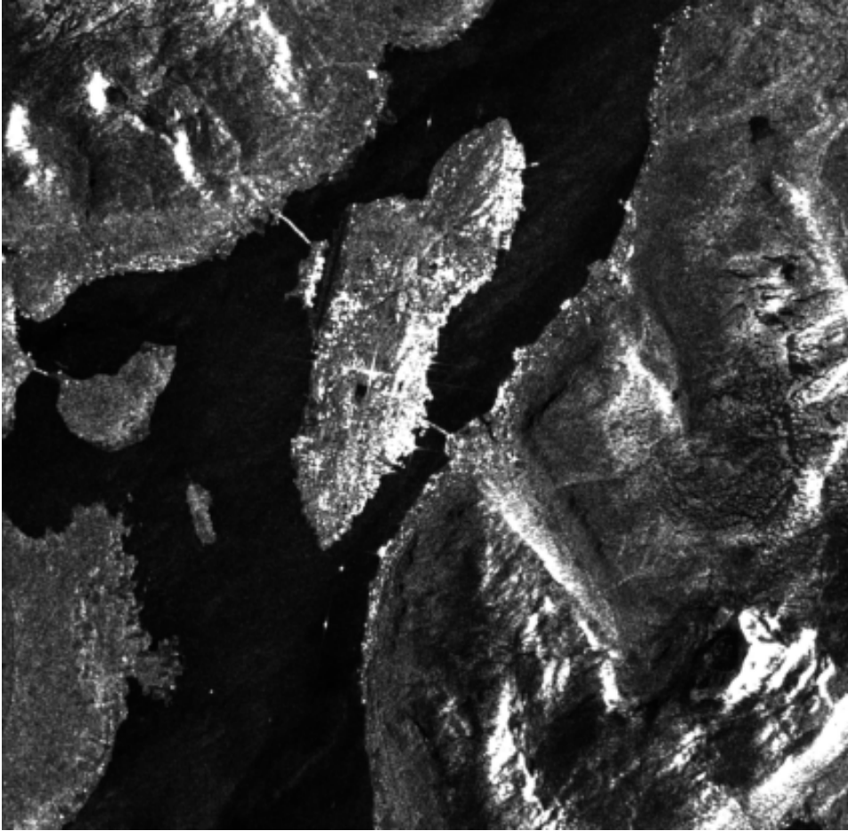
Figure 4.3: An example of a SAR image. This image shows the island of Tromsø. Looking at the bright points in the sea surrounding the island, it is clear how vessels can be easily detected using SAR with a cross-polarisation modality. This image was created from Sentinel-1 data using Sentinel Hub API 1 .
