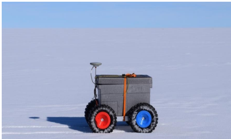
Figure 5. The 'CIC' rover is the type of platform that could be used with ice-penetrating radar for archaeological surveys to search for former bases that have been covered and associated equipment, such as aircraft within the ice (CIC Project).
