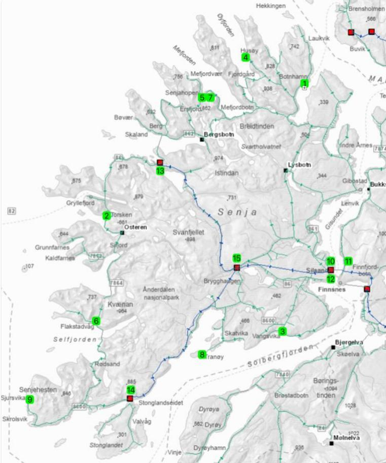
Figure 4-1 A map of the model area where zones are marked with numbers. Zones 1-10 are load nodes, while zones 11-15 are junction nodes.
